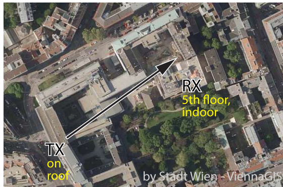
Fig. 4. Bird's eye view of the measurement scenario. The two X-pol antennas of the BS are located on a roof approximately 150 m away from the indoor receiver in downtown Vienna, Austria.
