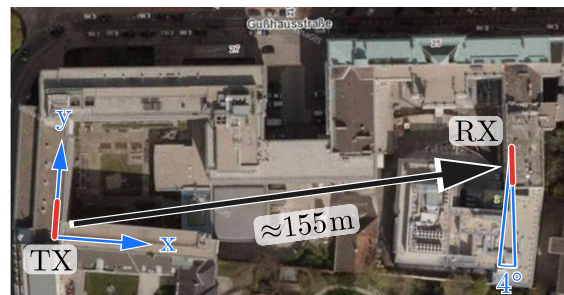
FIGURE 1. Aerial photograph of the measurement scenario at TU Wien [29]. The red lines indicate the orientation of the antenna arrays. The coordinate system orientation is indicated in blue.
