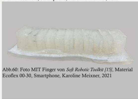
Abb.60: Foto MIT Finger von *Soft Robotic Toolkit* [15], Material Ecoflex 00-30, Smartphone, Karoline Meixner, 2021
