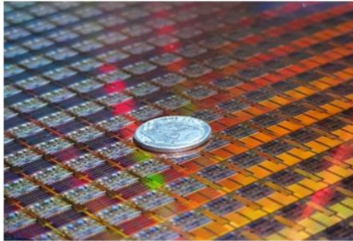
Fig.1.2: A wafer with several Intel processors with each processor, smaller than a dime, containing several hundreds of millions of transistors, invisible to the naked eye.
