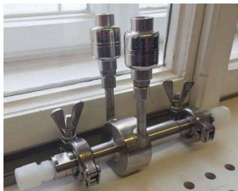
Figure 7 (left) and Figure 8 (right): Gassing devices, vortex on the left and sparger on the right
