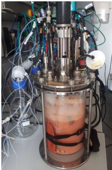
Figure 13 (left) and Figure 14 (right): Individual reactor vessel on the left and view on the multi-port head plate on the right
