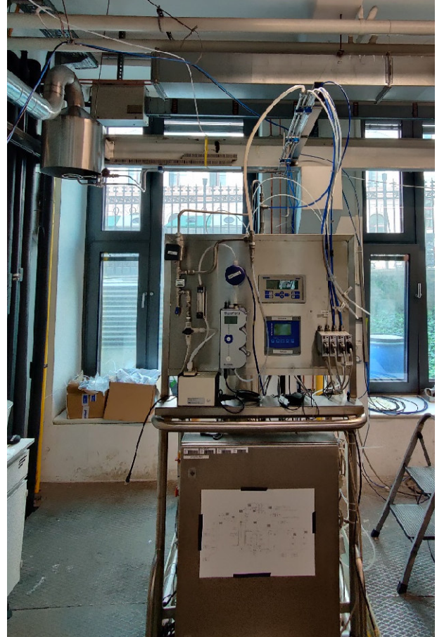
Figure 5 (left) and Figure 6 (right): BCR setup with view from the back on the left and view from the front on the right, the combustion hood can be seen in the top left corner
