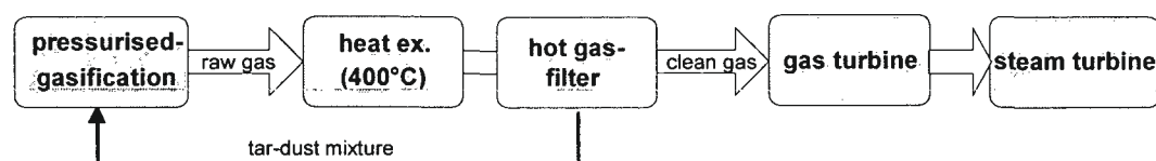
Fig. 4-3: Process scheme of concept I
