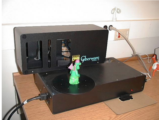
Figure 3.6: Cyberware Desktop 3D Scanner Model 15 [16].
