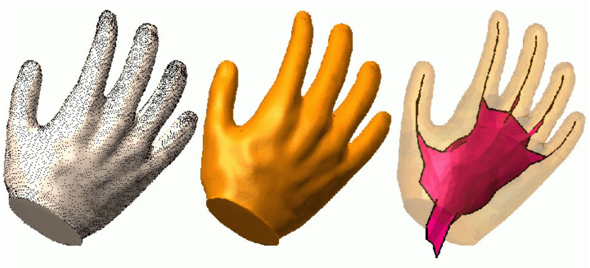
Figure 8.1: A set of input points from the surface of an object, the watertight output mesh, and a simplified version of the approximate inner-medial axis [42].
