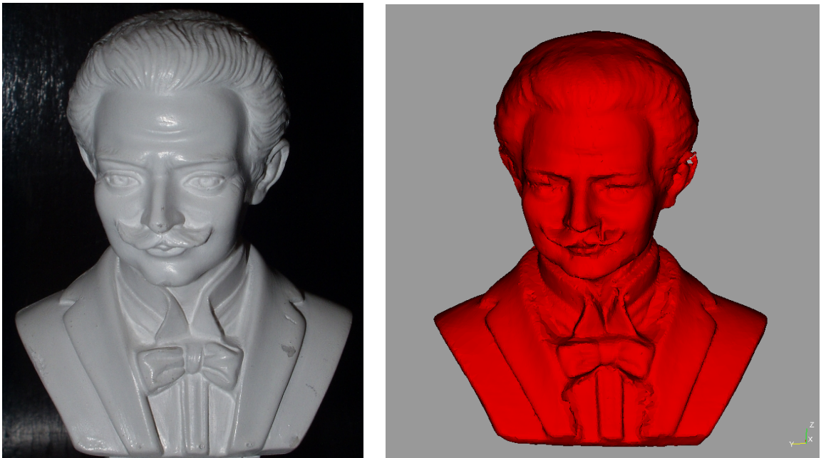
Figure 10.5: Photograph of the gypsum bust (height \sim 100 mm) (left), final reconstruction after Decimation and Smoothing (right).
