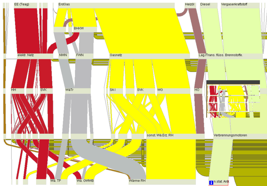
Figure 2.16: The energy distribution in a city visualized using an interactive Sankey diagram. Different types of energy are represented by the nodes, and the width of nodes as well as edges provides information about the quantitative flow of energy. Image courtesy of Riehman et al. [56]
