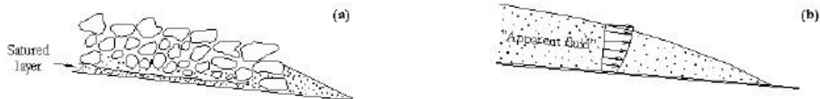
Figure 2.4 a. Prototype of a heterogeneous and complex moving mass; b. A homogeneous "apparent fluid" replaces the slide mass (HUNGR, 1995)
