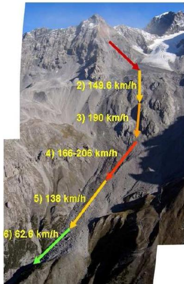
Figure 5.2 The velocities of the detached mass at several regions acquired from the movie shot on actual event (SOSSIO & CROSTA, 2007)
