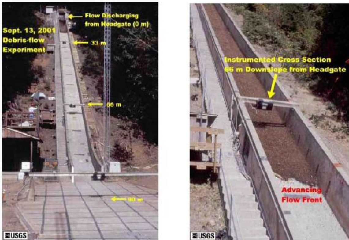
Figure 2.1 a. A debris flow discharging from the gate at the head of the flume. b. Debris flow passing instrumented cross section. (Images courtesy of U.S. Geological Survey)
