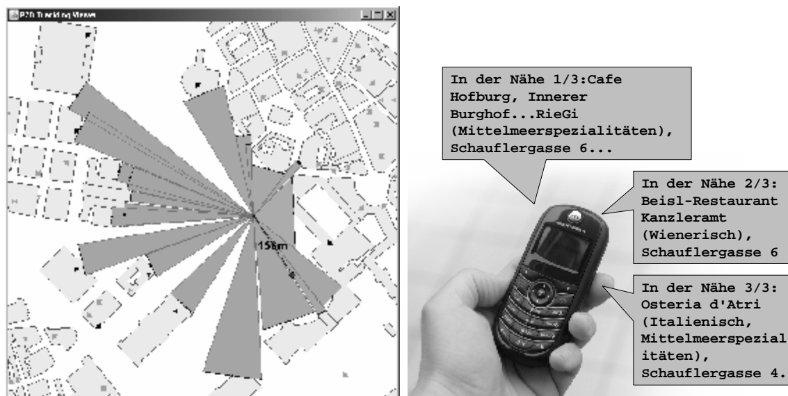
Figure 63. LVis query result and corresponding SMS response (Heldenplatz)
