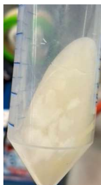
Figure 30: [EMIM]Cl with 2wt% PHB after centrifugation. In contrast to dissolving BM, the IL with PHB solidifies. PHB has probably settled on the surface (white spots).
