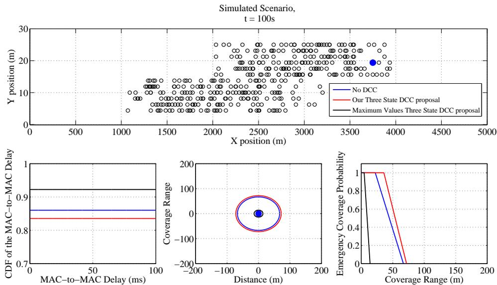
Figure 5.22: Simulation Results for a Vehicle initialized in *Restrictive State*( $t=100$  s)
