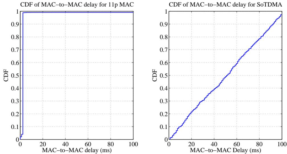
Figure 5.6: Empirical CDF of MAC-to-MAC delay of all correctly decoded packets for 100 ms deadline in lightly-loaded scenarios (50 vehicles)
