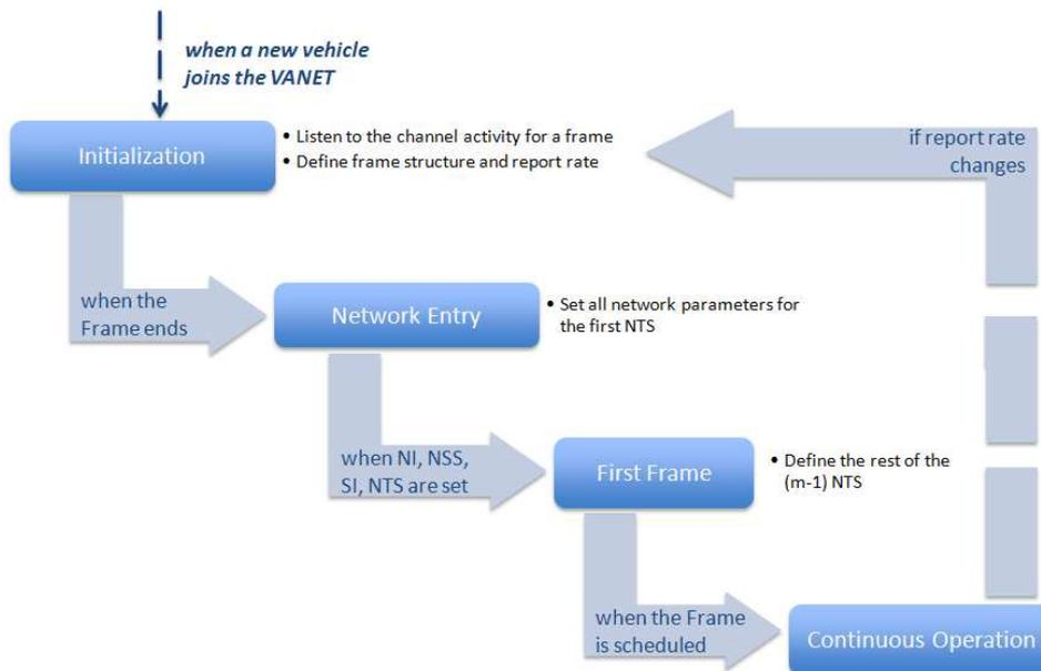
Figure 3.1: Flow chart of the SoTDMA MAC Protocol
