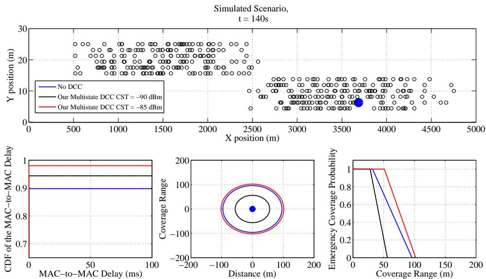
Figure 5.36: Simulation Results for a Vehicle initialized in *Relaxed State* ( $t=140$  s) for CST-85 dBm
