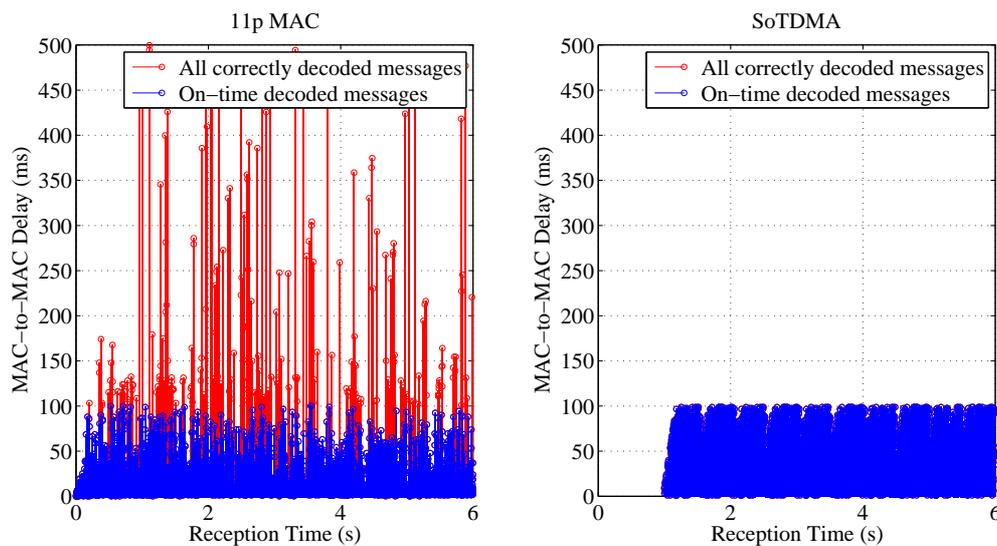
Figure 5.7: MAC-to-MAC delay of all correctly decoded packets vs. reception time for heavily-loaded scenarios (400 vehicles)
