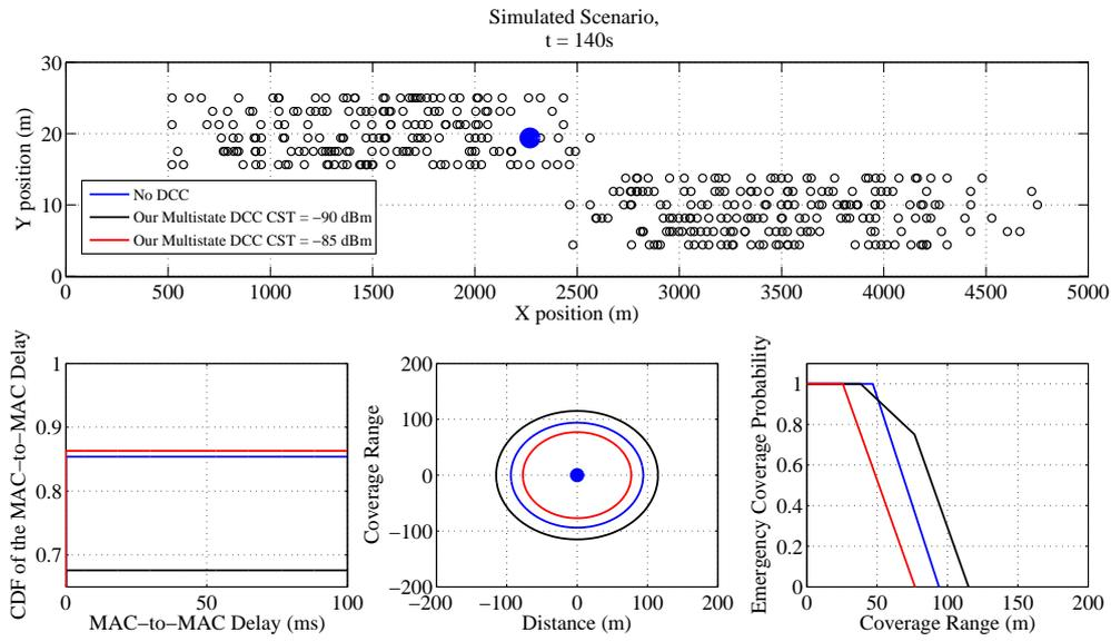
Figure 5.37: Simulation Results for a Vehicle initialized in *Restrictive State* ( $t=140$  s) for  $CST=85$  dBm
