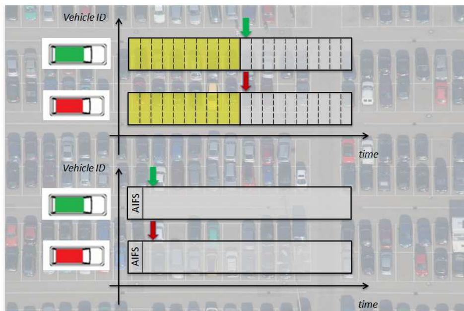
Figure 5.4: Several vehicles turned on during one frame duration might attempt to gain channel access at the same time due to the same perception of the frame (unintended slot reuse)
