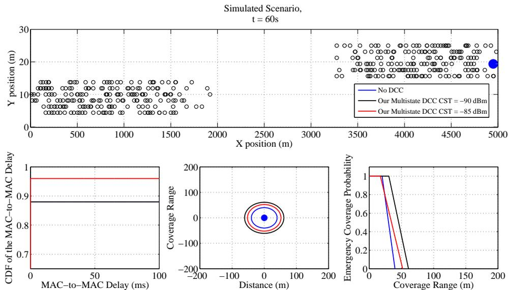
Figure 5.33: Simulation Results for a Vehicle initialized in *Restrictive State* ( $t=60$  s) for CST-85 dBm
