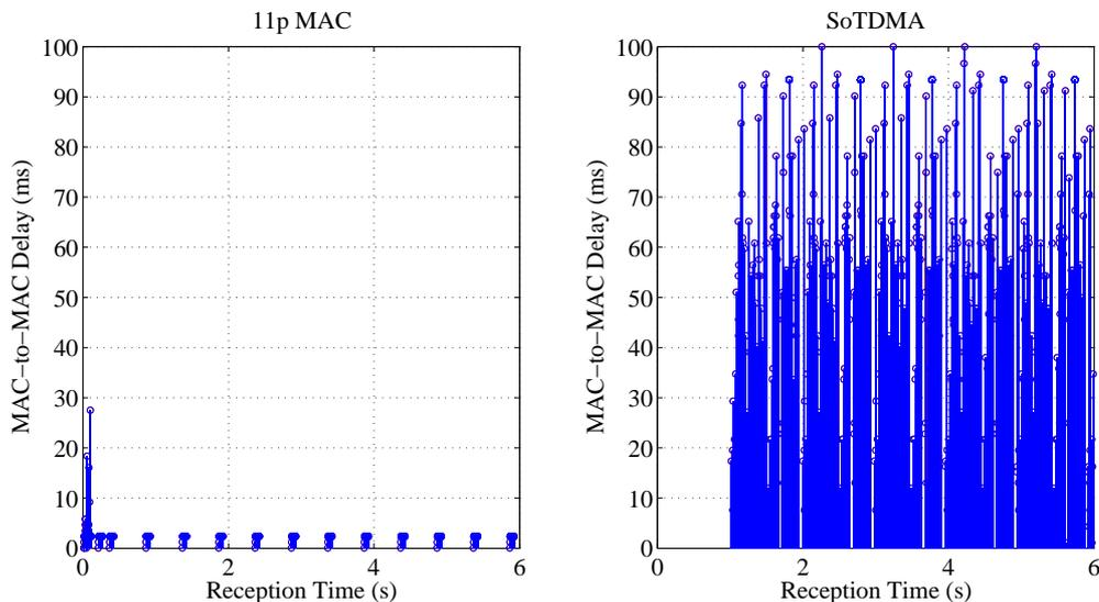
Figure 5.5: MAC-to-MAC delay of all correctly decoded packets vs. reception time for lightly-loaded scenarios (50 vehicles)
