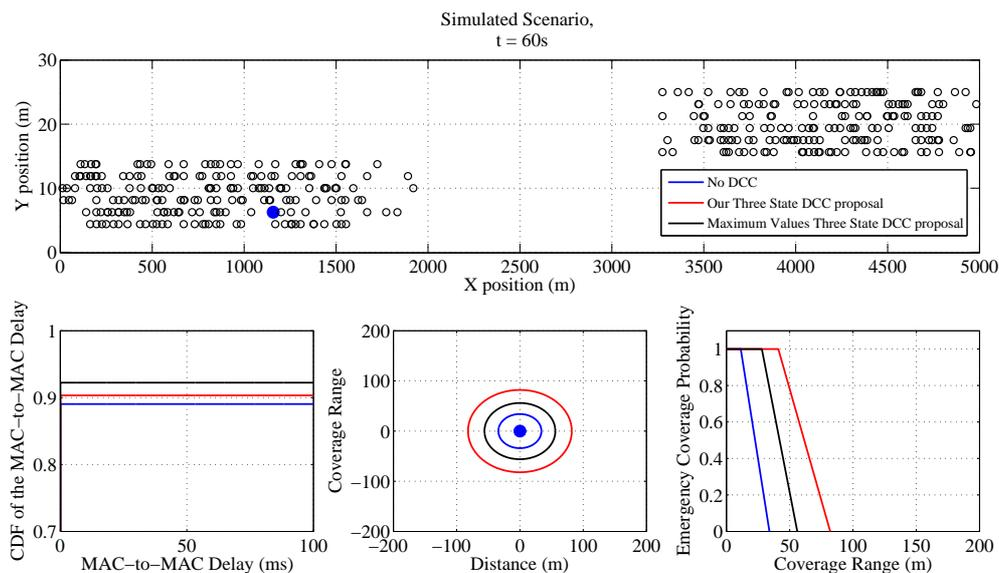
Figure 5.19: Simulation Results for a Vehicle initialized in *Relaxed State* ( $t=60$  s)
