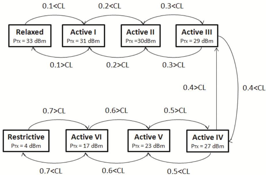
Figure 5.26: Multistate active DCC Mechanism design for  $CST = -90$  dBm
