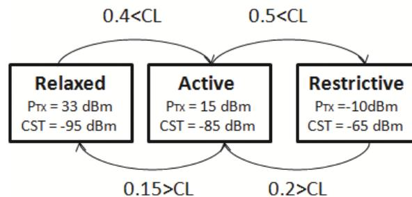
Figure 5.14: Three-State Maximum Values DCC Mechanism design
