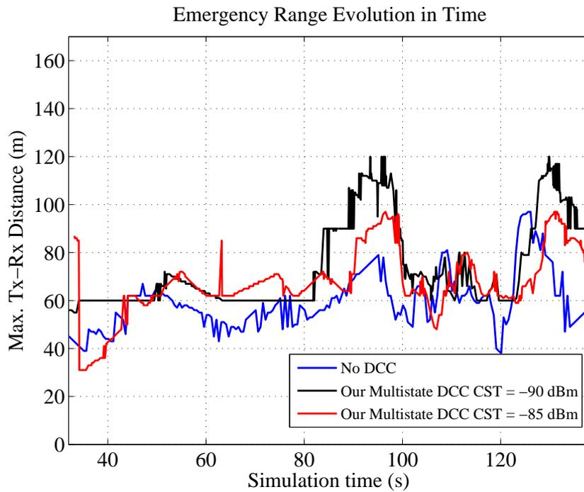
Figure 5.30: Emergency Range vs Simulation Time for a Vehicle initialized in *Active State* for  $CST = -85$  dBm
