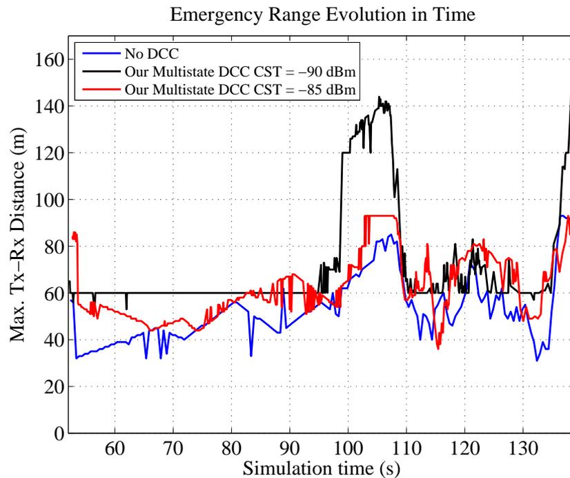
Figure 5.31: Emergency Range vs Simulation Time for a Vehicle initialized in *Restrictive State* for  $CST=-85$  dBm
