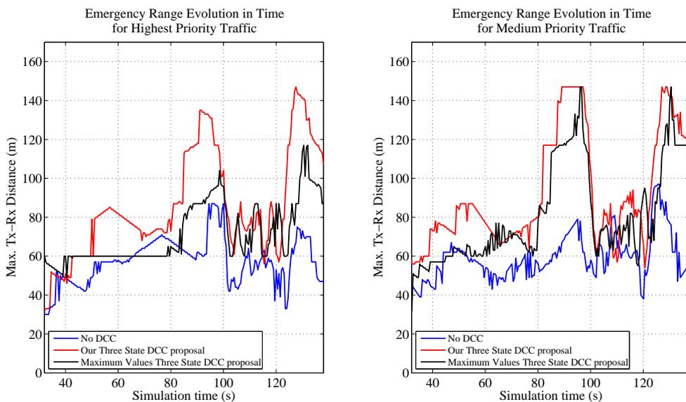
Figure 5.17: Emergency Range vs Simulation Time for a Vehicle initialized in *Active State*
