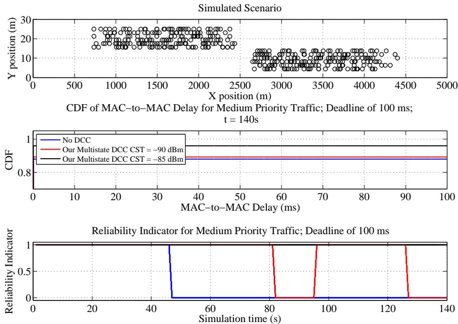
Figure 5.38: System Performance for two VANET merging scenario: CDF of MAC-to-MAC Delay and Reliability Indicator for  $CST = -85$  dBm
