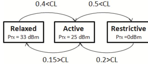
Figure 5.15: Three-State Our DCC Mechanism design for  $CST = -90 \text{ dBm}$
