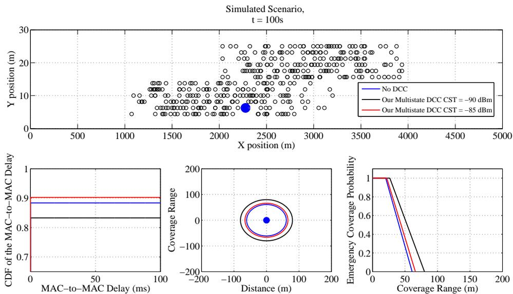
Figure 5.34: Simulation Results for a Vehicle initialized in *Relaxed State* ( $t=100$  s) for CST $-85$  dBm
