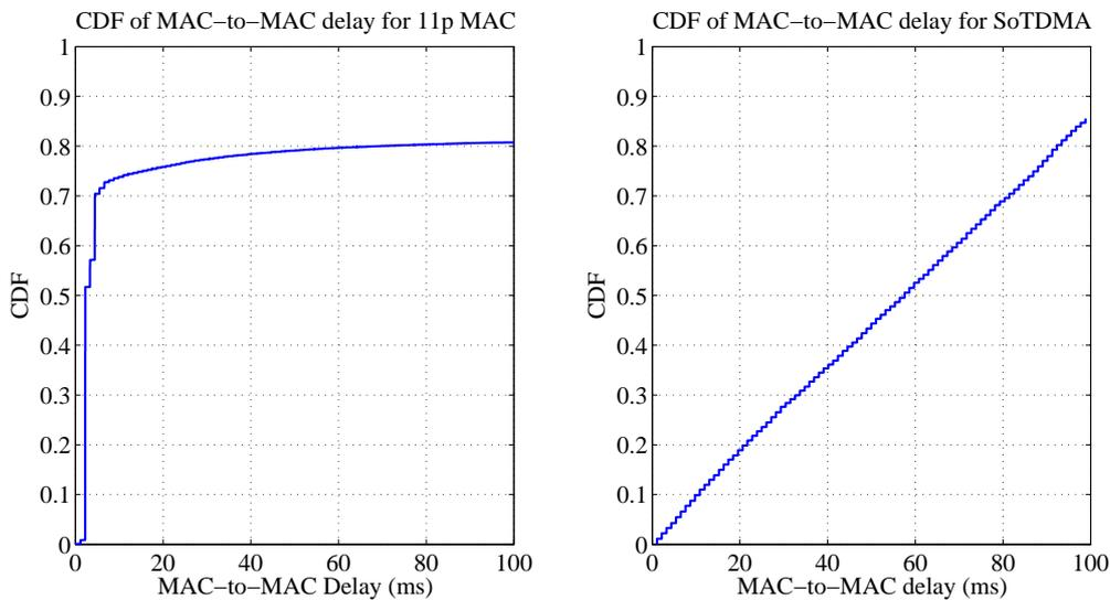
Figure 5.8: Empirical cumulative distributed function of MAC-to-MAC delay of all correctly decoded packets for 100 ms deadline in heavily-loaded scenarios (400 vehicles)
