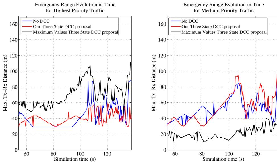
Figure 5.18: Emergency Range vs Simulation Time for a Vehicle initialized in *Restrictive State*
