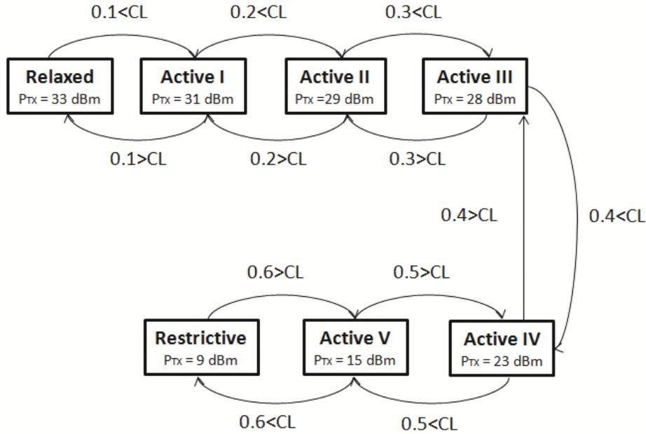
Figure 5.28: Multistate active DCC Mechanism design for  $CST=-85$  dBm
