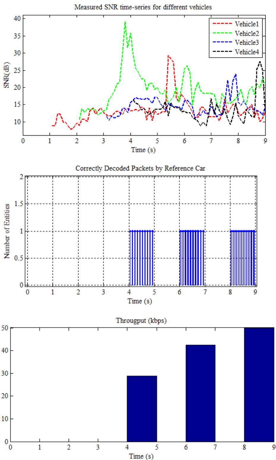
Figure 5.3: Channel structure, Measured SNR time-series for different vehicles, Correctly Decoded Packets and Throughput for a car driving along in the scenario
