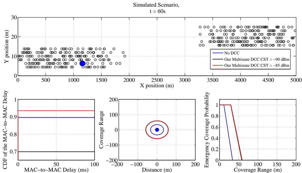
Figure 5.32: Simulation Results for a Vehicle initialized in *Relaxed State* ( $t = 60$  s) for  $CST = -85$  dBm
