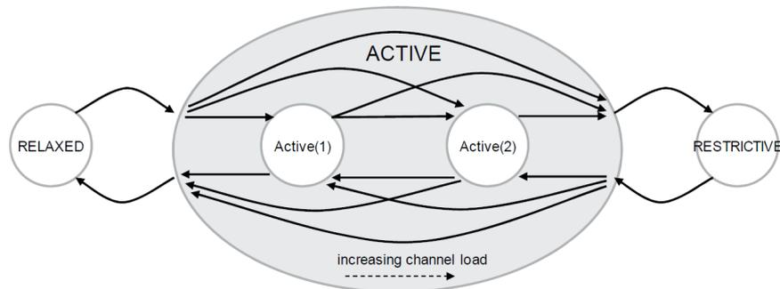
Figure 3.2: Currently proposed DCC Mechanism: The state machine proposed by ETSI DCC framework (ETSI TS 102 687 V1.1.1 (2011-07))
