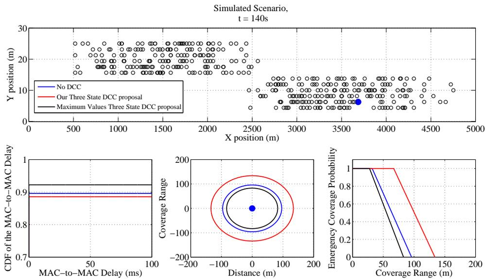
Figure 5.23: Simulation Results for a Vehicle in initialized in *Relaxed State*( $t=140$  s)
