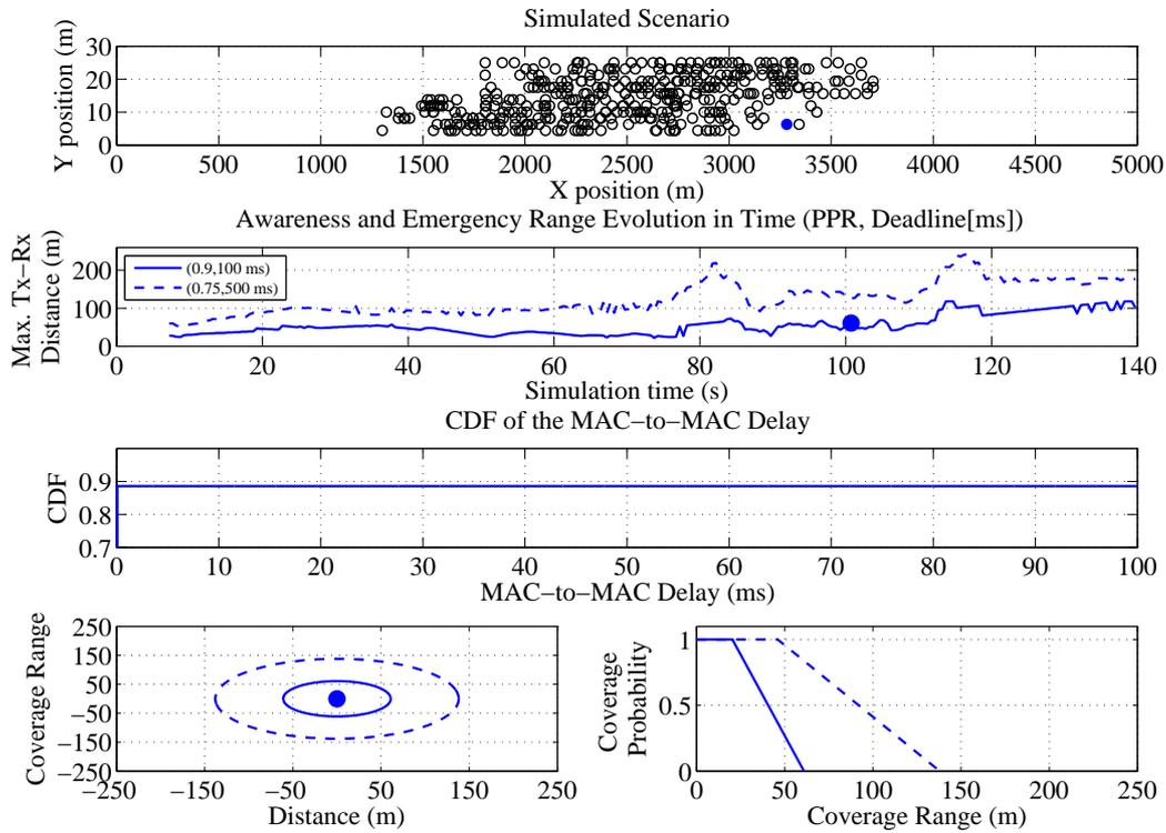
Figure 5.13: Simulation Results for a Vehicle in Relaxed State
