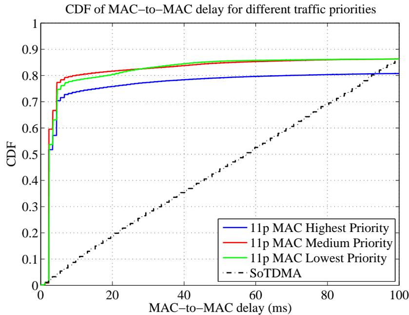
Figure 5.9: Empirical CDF of MAC-to-MAC delay of all correctly decoded packets for 100 ms deadline in heavily-loaded scenarios (400 vehicles) for different priorities
