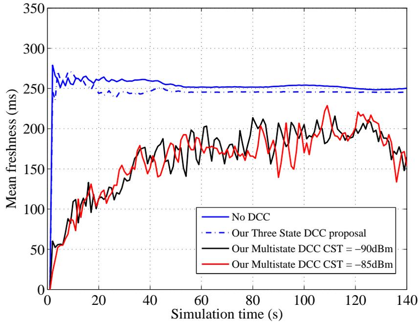
Figure 5.39: System Performance for two VANET merging scenario: Mean Freshness
