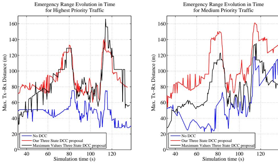
Figure 5.16: Emergency Range vs Simulation Time for a Vehicle initialized in *Relaxed State*
