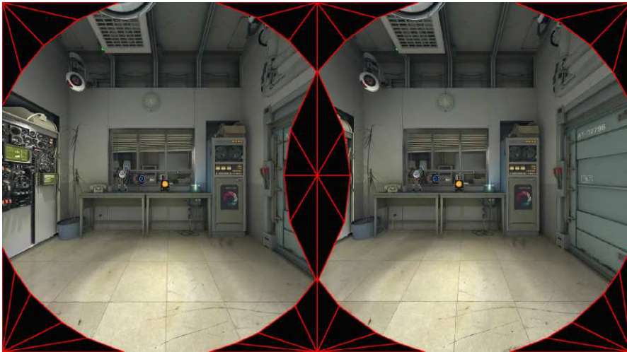
Figure 2.21: Simplified mesh to approximate the areas where pixels from the displays are not visible to a user due to the optics. The hole in the middle corresponds to the region which is typically occluded by the nose. Reprinted from [Vla15].
