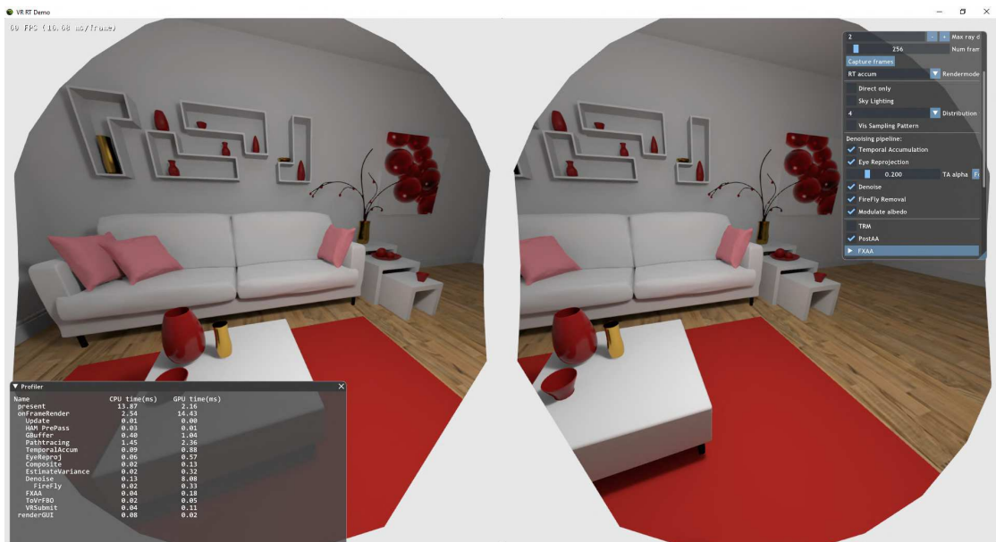
Figure 4.1: Screen shot of prototype application. The current view displayed in the plugged in HMD is mirrored. On top, a simple UI is rendered for parameter tweaking and profiling.
