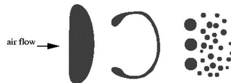
Figure 5: Schematic illustration of the bag breakup [2]
