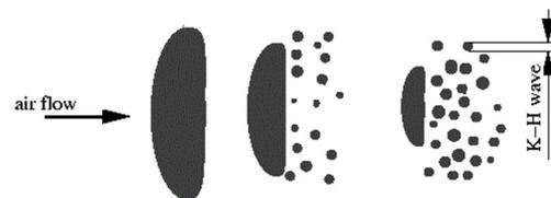
Figure 6: Schematic illustration of the s-t breakup [2]
