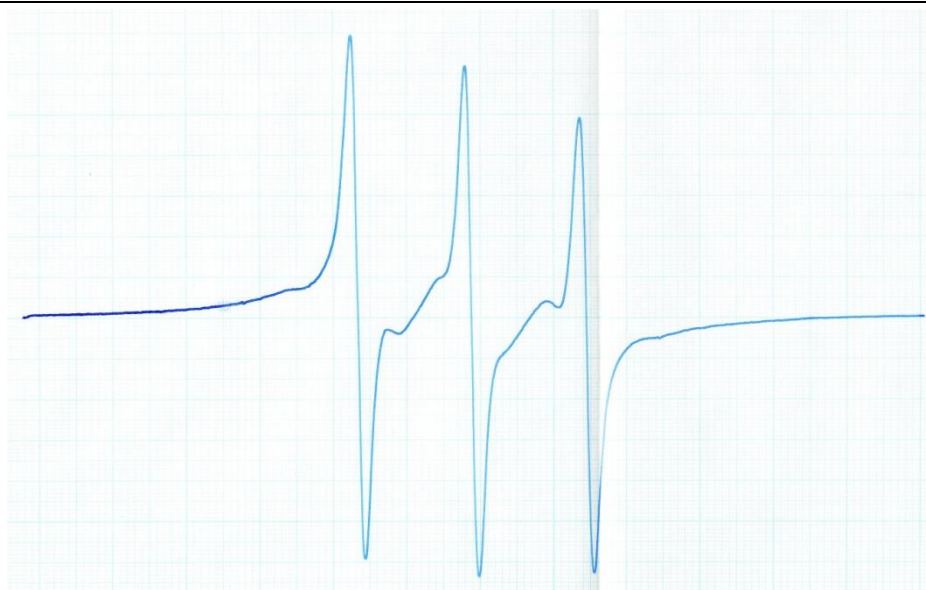
Figure 40: First ESR measurement with the additional smaller peaks as indication for a successful synthesis of R2cS1
