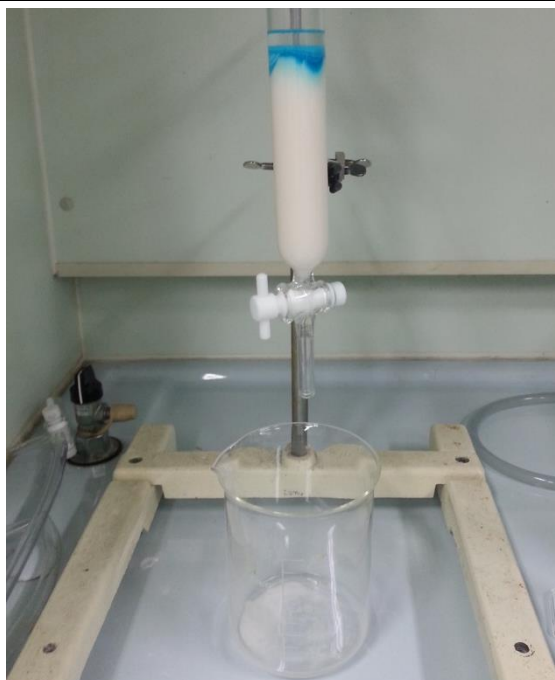
Figure 41: Removing TEMPOL from the reaction solution by flushing the product mixture with \text{HCCl}_3 in \text{AlO}_3 gel
