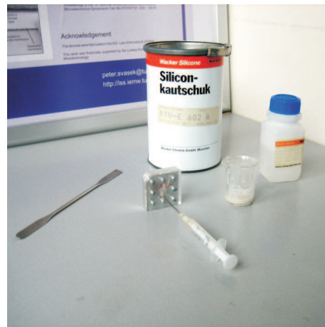
Figure 4.13: Injecting the liquid silicone mixture by means of a conventional medical-syringe into the mould. The mould is kept in an upright position for curing to allow air bubbles leaving the mould through the drain.
