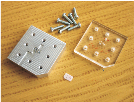
Figure 4.12: Top view of the disassembled mould. The PMMA cover, the milled Al-body and metal pins define the geometry of the Silicone gasket. A moulded gasket lies in front of the other parts. See also Fig. 7.5.
