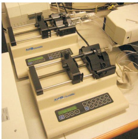
Figure 5.2: The KDScientific Model 200 syringe pumps allow to drive two syringes at once.
