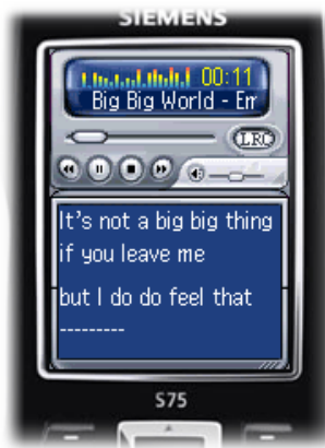
Figure 2.2: LyricShow Player: A audio player programmed in J2ME showing the lyrics while playing the song
