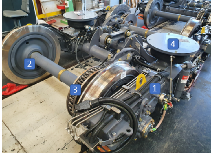
Figure 2.5: A non-driven bogie from the head car. The main components are numbered as follows; (1) bogie frame, (2) wheel and axle, (3) brake disc, (4) air suspension.
