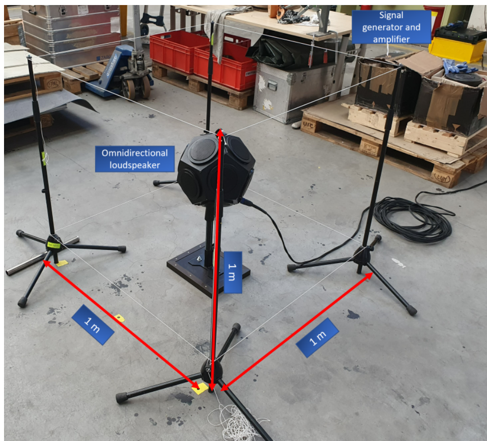
Figure 3.1: Setup for sound power measurement.
