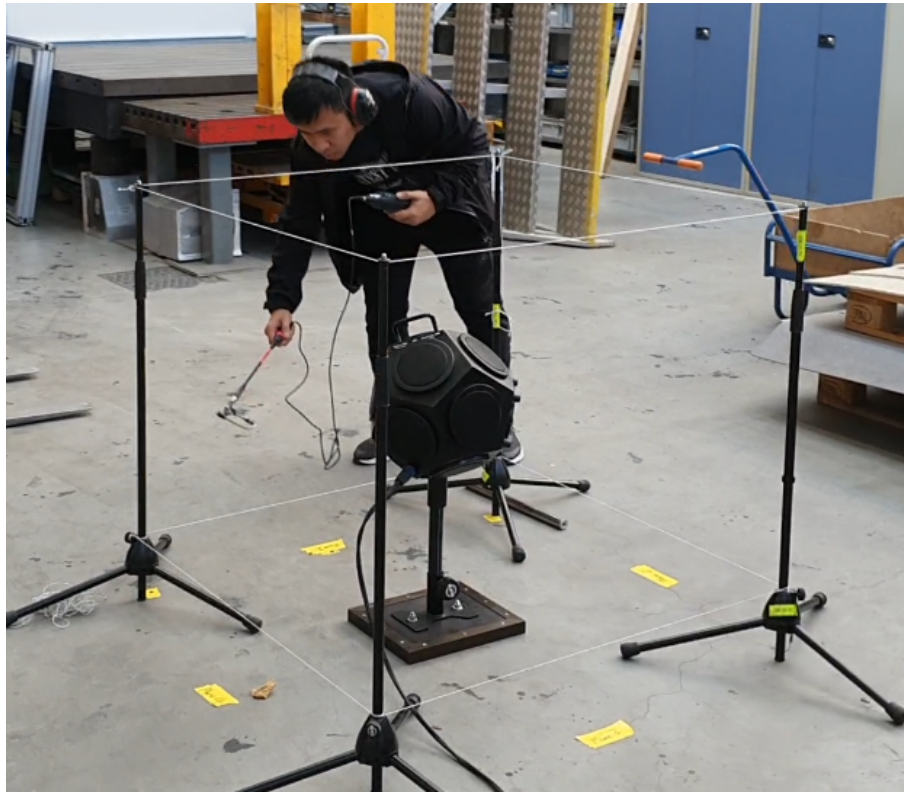
Figure 3.3: Intensity measurement using the two-microphone method according to ISO 9614-2 [5].
