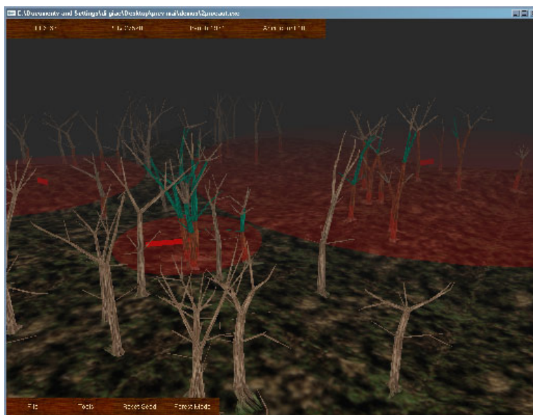
Figure 2.3: An Interactive Forest (Illustration from Giacomo [GCF01]). Red discs are wind influence objects; red branches are selected for animation; green ones transition between animated and static.
