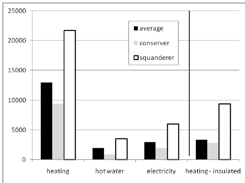
Fig. 12 Energy demand of hypothetical 3-persons households for heating (before and after insulation), hot water preparation, and electricity per year.
