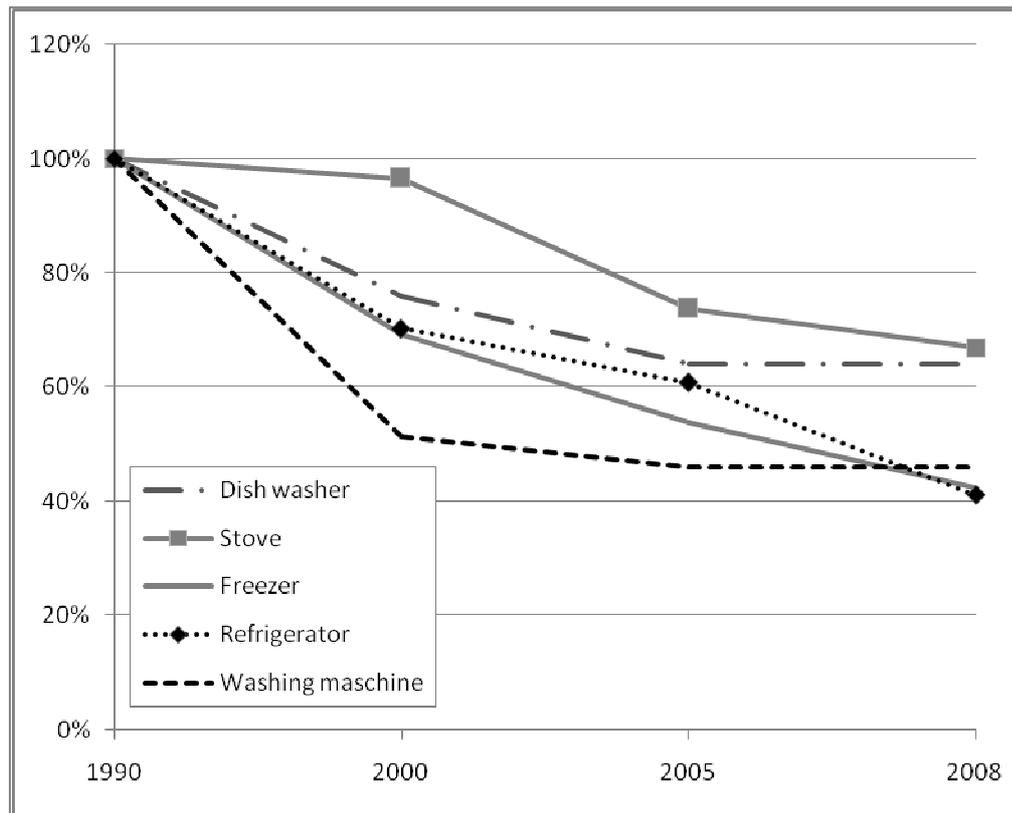
Fig. 7: Efficiency gains of different electrical household appliances between 1990 and 2008. Data source: Forum Haushaltgeräte 2008
