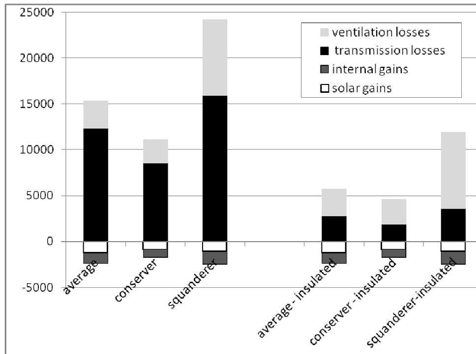
Fig. 14: Contribution of transmission and ventilation losses, solar and internal gains to the theoretical heating demand of the three household types. Gains are on the negative scale, losses on the positive scale, as it refers to resulting heating demand.
