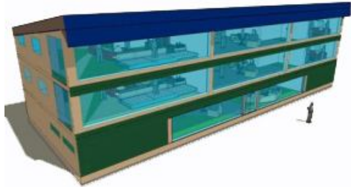
Figure 25 – Total front roof area available for PV modules (dark blue)
