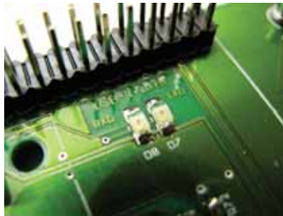
Figure 4.14. UART traffic LEDs of node 0
