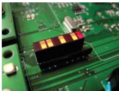
Figure 4.8. Bargraph connected to node 1
