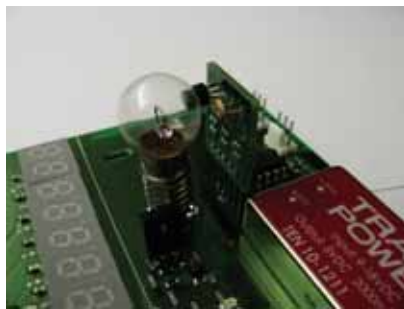
Figure 4.9. Light bulb with sensor PCB
