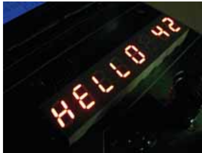
Figure 4.11. Seven–segment display connected to node 2
