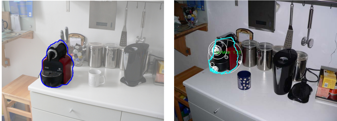
(a) One of the learning images for the coffee maker, the manually segmented region of interest is shown in blue. (b) Detecting the coffee maker with interest points.
