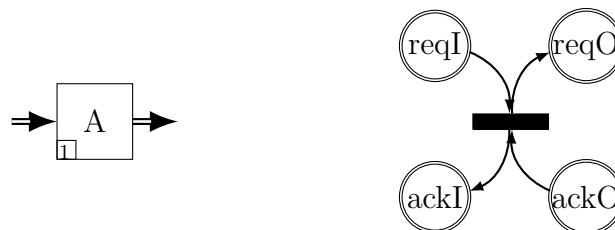
Figure 4.13: Bounded Queue Module of size 1
