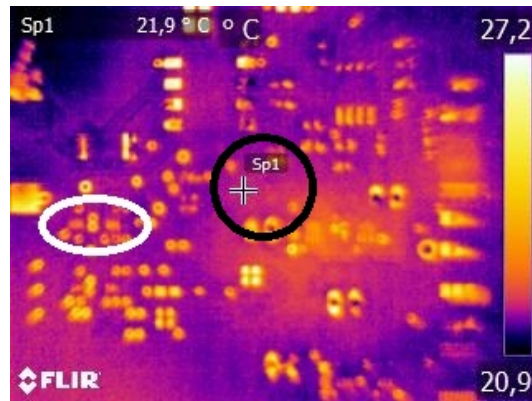
Figure 3.8: PCB temperature at 100 kHz switching frequency. GaN FETs are marked by a white ellipse, and the driver by the black circle.
