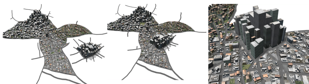
Fig. 2.11: Renderings of two urban layouts merged using graph cut. From left to right: (1) Two separated layouts (2) merged scene (3) closeup of merged areas. Image courtesy of Lipp et al. [LSWW10]
