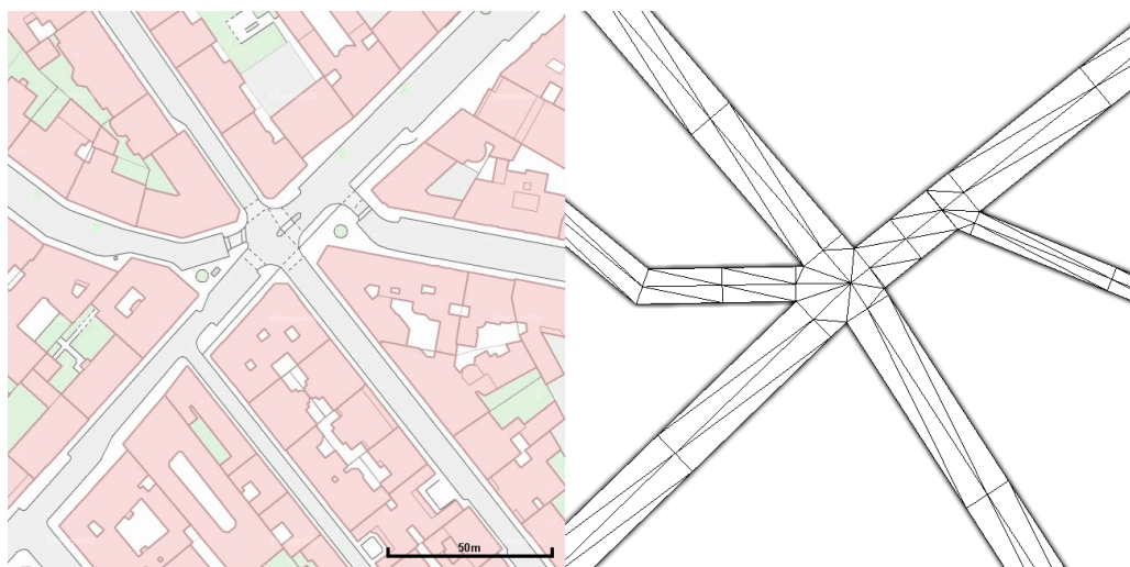
Fig. 5.1: Complex junctions connecting more than 4 street segments. Left: A crossing in the 4th district in Vienna (©ViennaGIS). Right: A similar junction modeled in my application.
