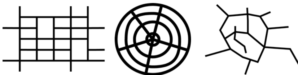
Fig. 4.1: Different street patterns. From left to right: (1) Grid/raster pattern (2) Radial/circular pattern (3) Organic pattern
