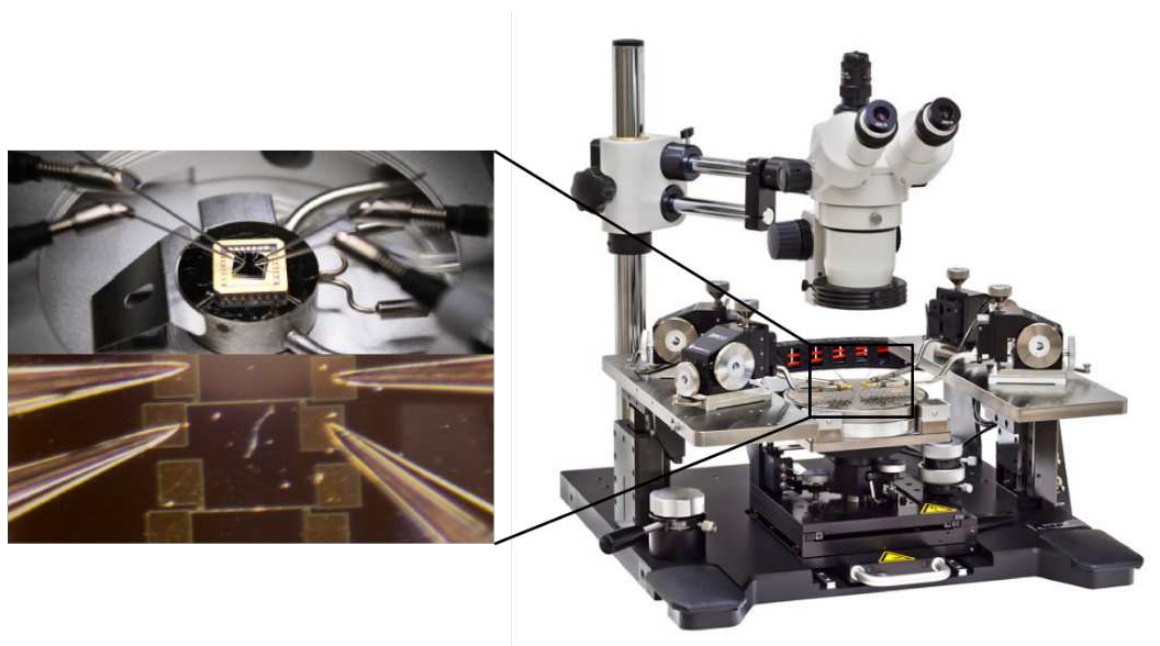
Figure 2.2: Commercially available manual probe station with a detailed view of the probes/sample through the microscope [14, 15].
