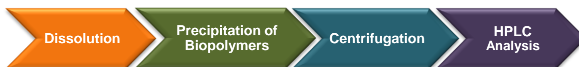
Figure 37: Working process for the extraction of Betulin from birch bark
