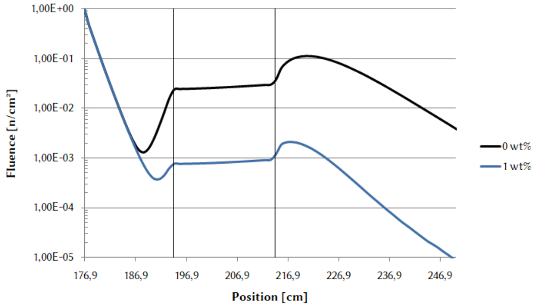
Fig. 38: Thermal neutron flux for 1 wt% boron compared to ordinary concrete
