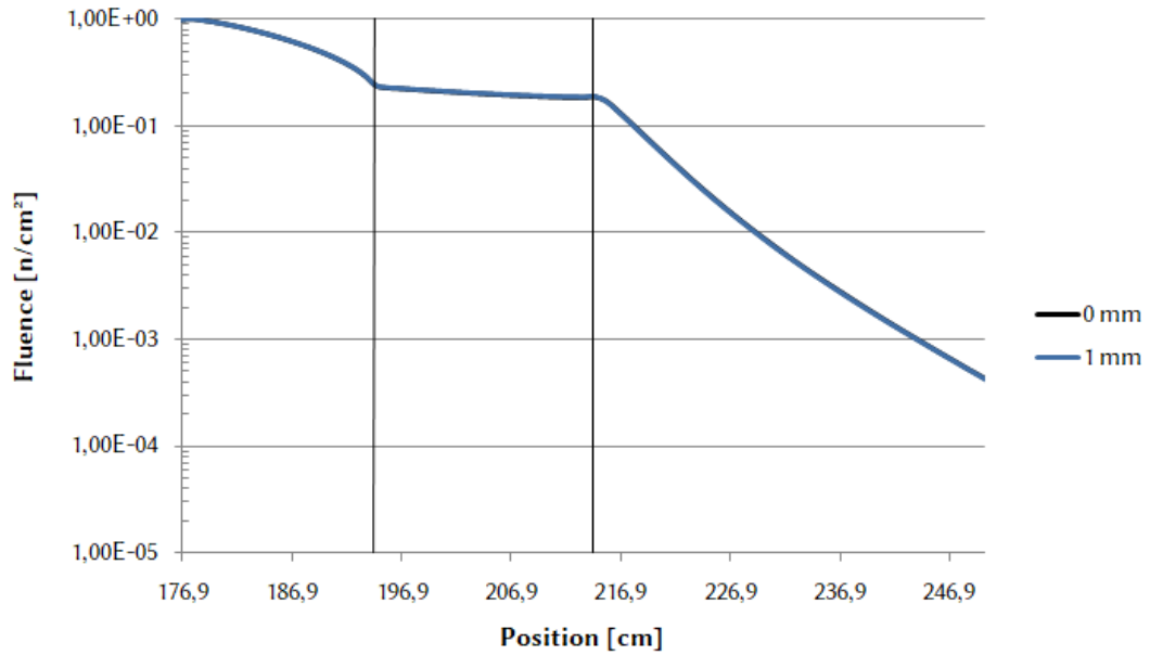
Fig. 47: Fast neutron flux for 1 mm cadmium cladding compared to standard shield
