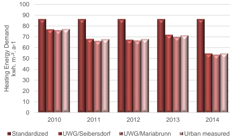
Figure 3-14 Heating demand for the apartment block using standardized, UWG-Seibersdorf, UWG-Mariabrunn compared to Innere Stadt observed weather
