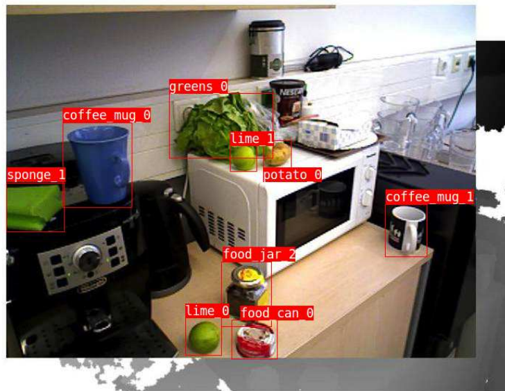
Figure 2.3: Example of an RGB-D frame from the Autonomous Robot Indoor Dataset with 2D bounding box annotation.
