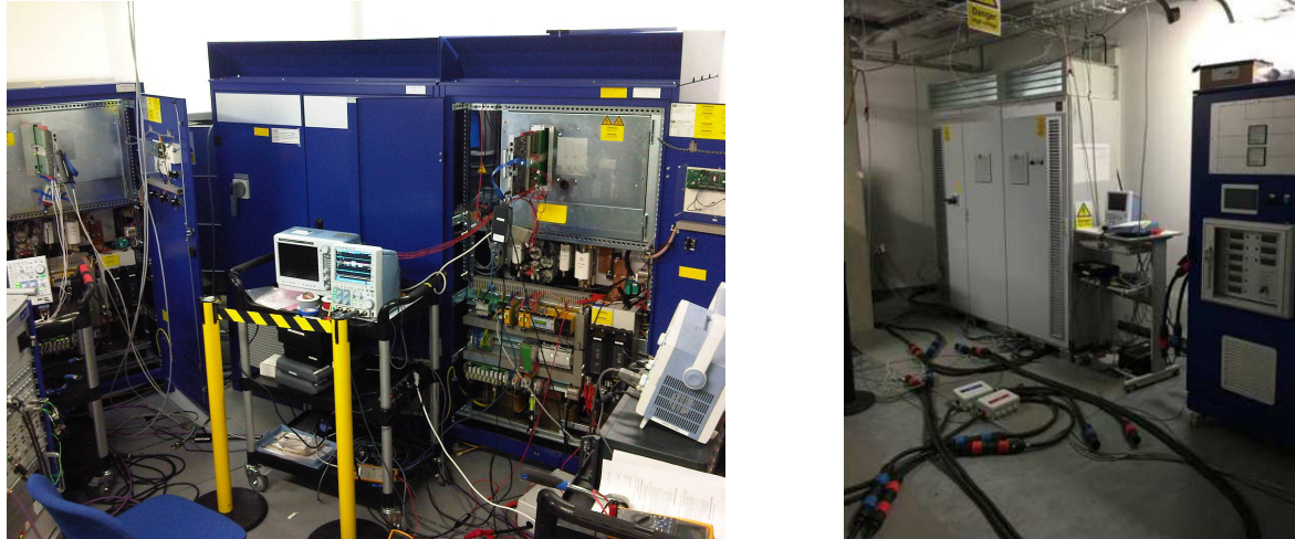
Figure 2.5: Battery emulator laboratory setup.
