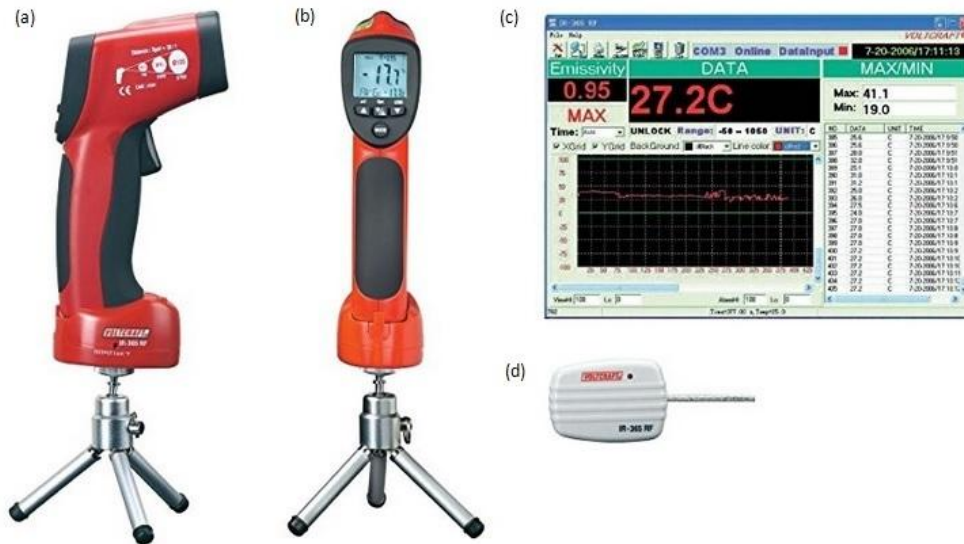
Figure 20: Overview and example of the VOLT CRAFT IR-365 RF infrared thermometer (a) side and (b) rear view (c) example of a measurement with the corresponding (d) wireless connection to the computer
