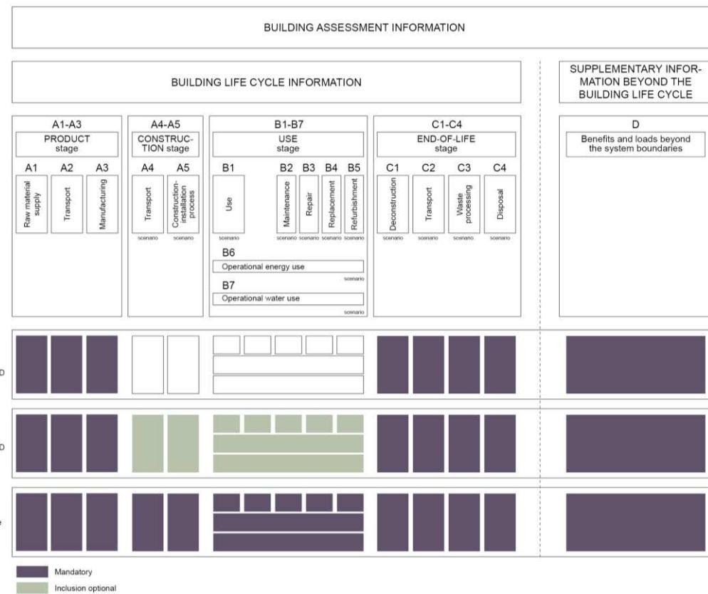
Figure 27. Life cycles stages to be included in an EPD according to EN amendment 15804:2018
