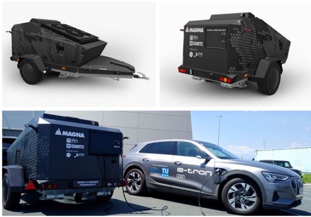
Fig. 3 MHP: CAD rendering of MHP and photo of MHP charging a BEV
