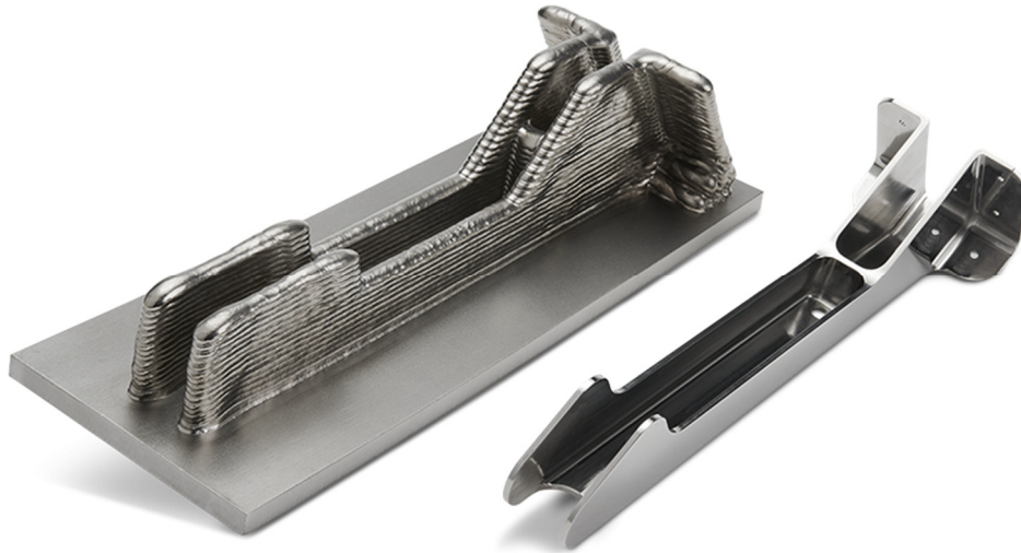
Figure 3: WAAM part for the Boeing 787 Dreamliner made by Norsk Titanium [3]
