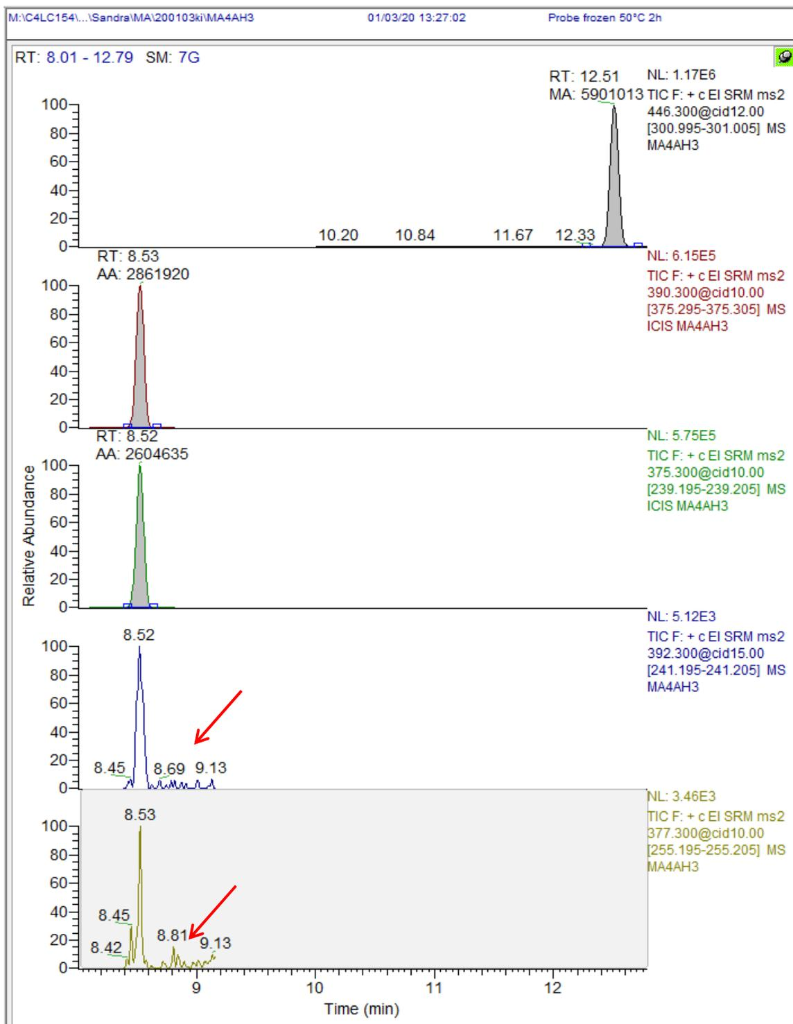
Figure 13: Preparation/analysis after freezing. Hydrolysis: Incubation 50 °C 2 hours. transitions for IS methyltestosterone (RT 12.51) and selected transitions for identification for **16** (RT 8.53) and **17** (RT 8.82) of a urine sample with **16** added as IS.
