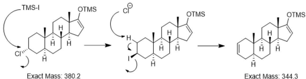
Scheme 8: Elimination process occurring during derivatization
