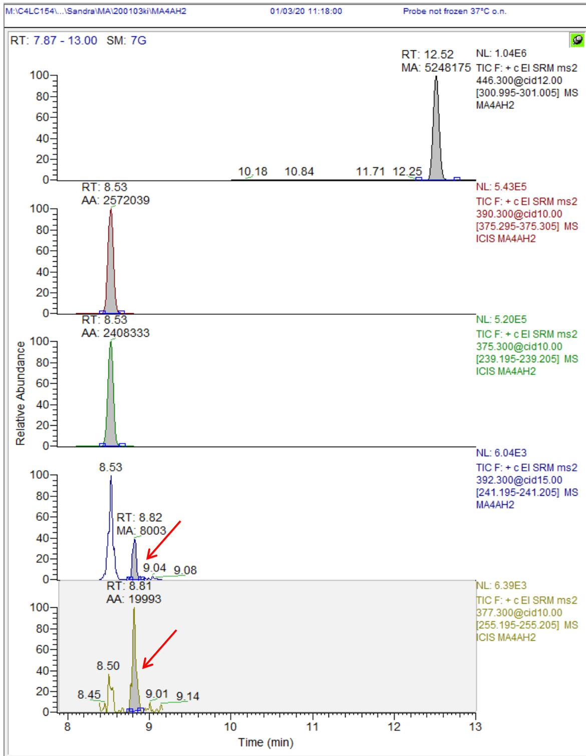
Figure 14: Preparation/analysis before freezing. Hydrolysis: Incubation 37 °C overnight. Transitions for IS methyltestosterone (RT 12.52) and selected transitions for identification for **16** (RT 8.53) and **17** (RT 8.82) of a urine sample with **16** added as IS.
