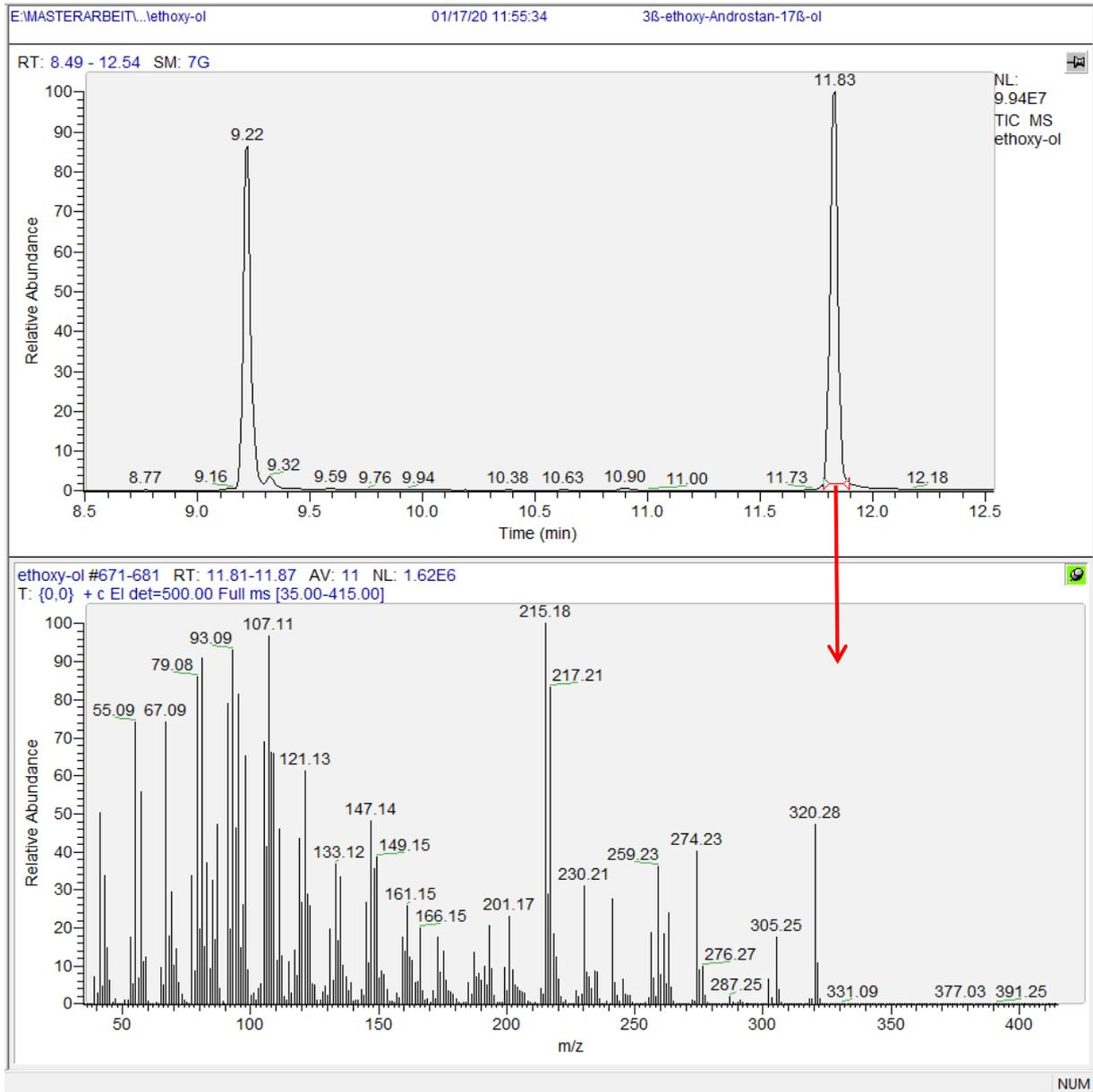
Figure 45: GC-MS chromatogram and full scan spectra of 17 without derivatization
