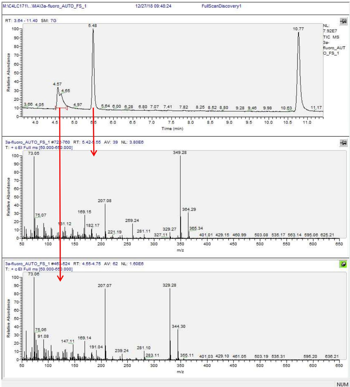
Figure 7: full scan chromatogram of internal standard *d3*-testosterone (RT 10.77), **14** (RT 5.48) and its elimination product (RT 4.57). The corresponding mass spectra for **14** and its elimination product are shown below.
