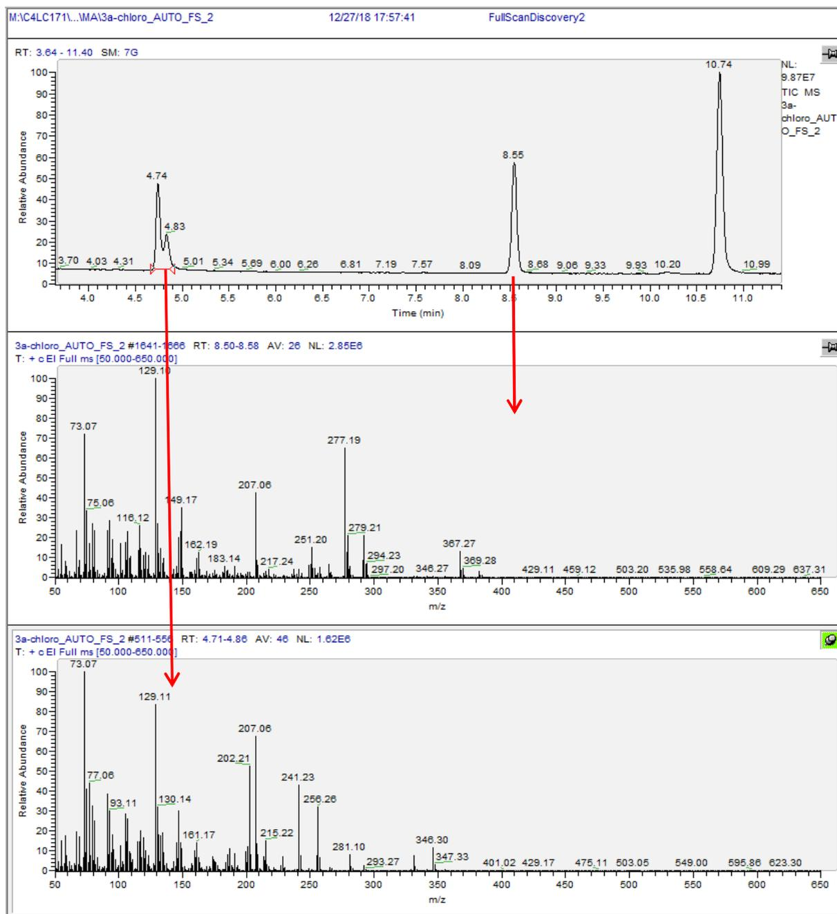
Figure 27: full scan chromatogram of internal standard d3-testosterone (RT 10.74), **13** (RT 8.55) and its elimination product (RT 4.74). The corresponding mass spectra for **13** and its elimination product are shown below.
