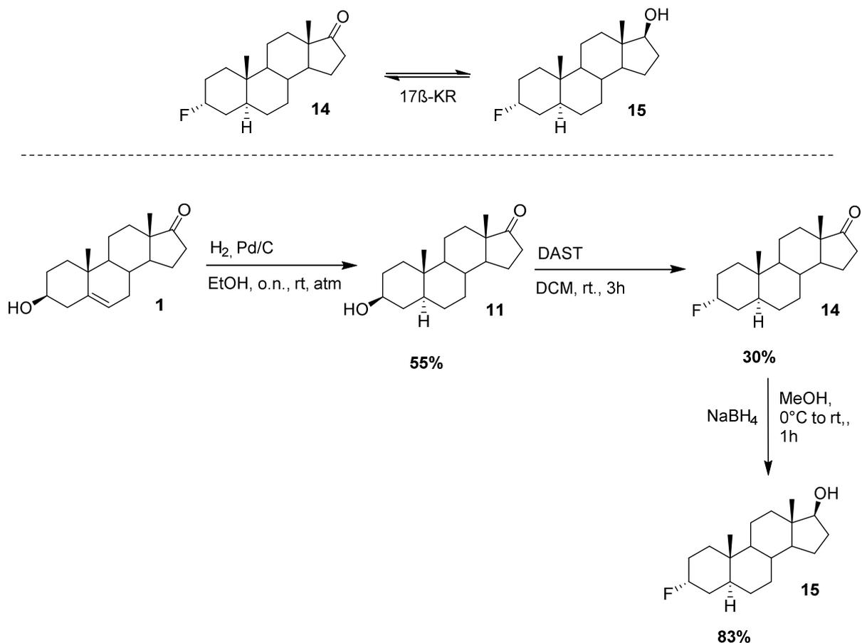
Scheme 9: synthetic route for 3 $\alpha$ -fluoro-5 $\alpha$ H-androstane-17-one and 3 $\alpha$ -fluoro-5 $\alpha$ H-androstane-17 $\beta$ -ol
