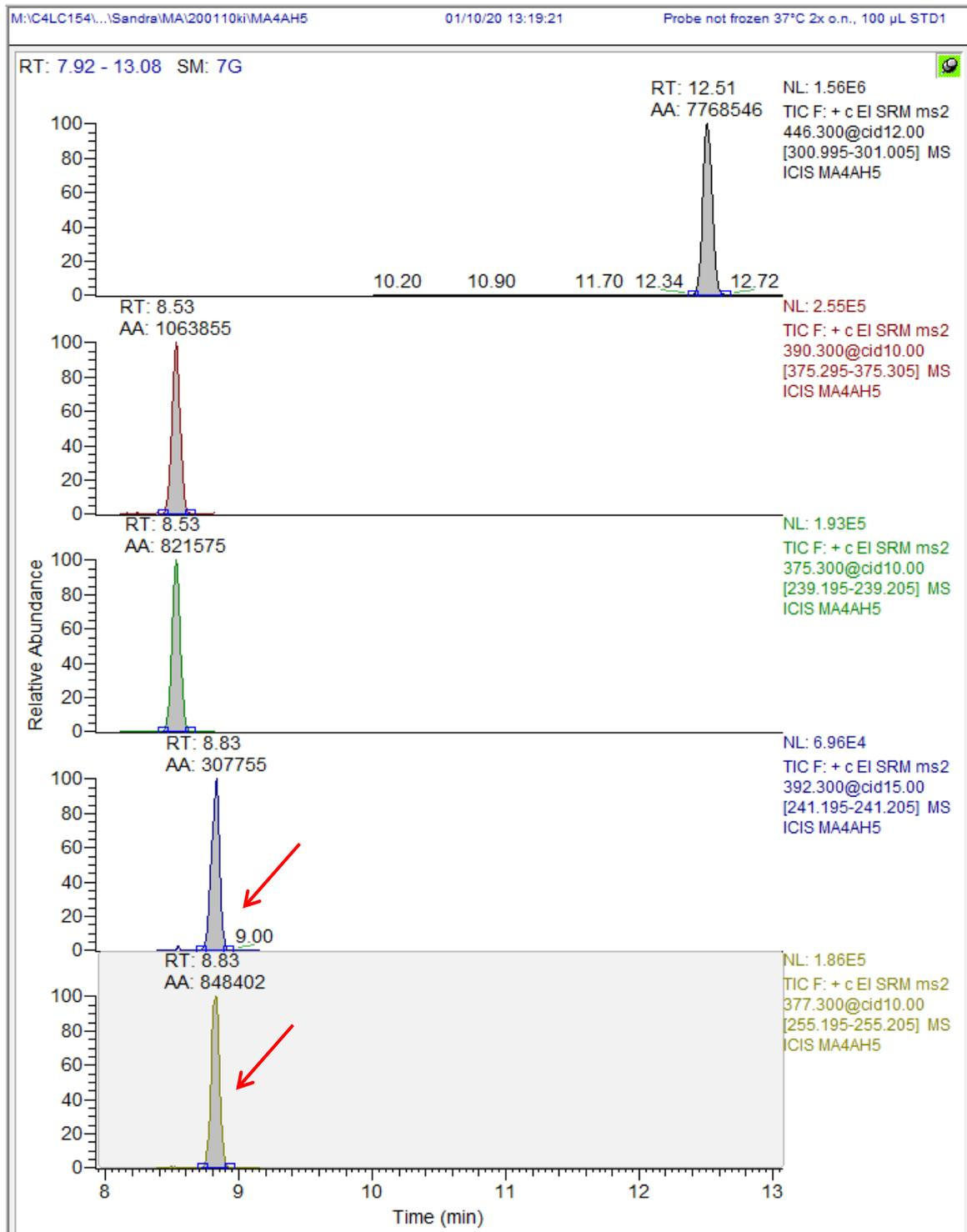
Figure 15: Preparation/analysis before freezing. Hydrolysis: Incubation 37 °C, **two** times overnight. Transitions for IS methyltestosterone (RT 12.51) and selected transitions for identification for **16** (RT 8.53) and **17** (RT 8.83) of a urine sample with **16** added as IS.
