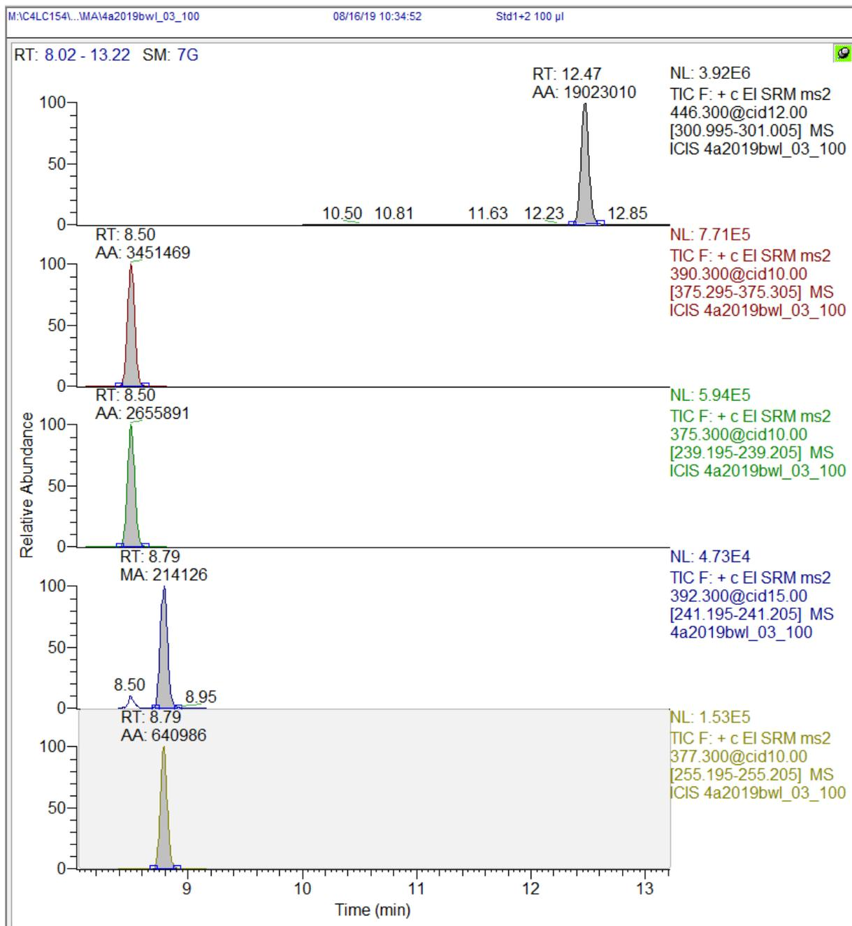
Figure 10: transition for IS methyltestosterone (RT 12.47) and selected transitions for identification for **16** (RT 8.50) and **17** (RT 8.79) of a urine sample spiked with **16** and **17**
