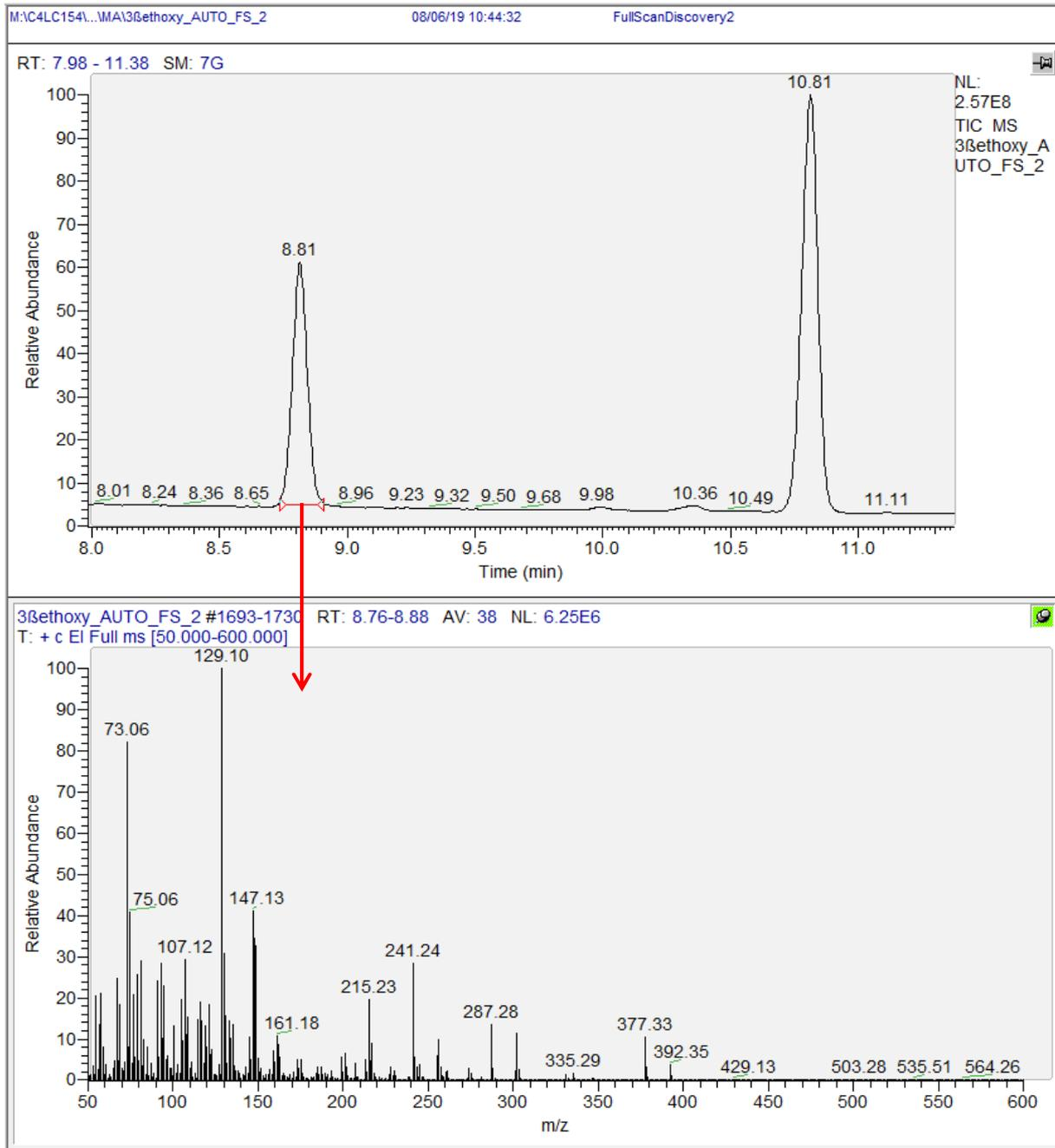
Figure 9: full scan chromatogram of IS d3-testosterone (RT 10.81) and **17** (RT 8.81). The corresponding mass spectrum for **17** is shown below.
