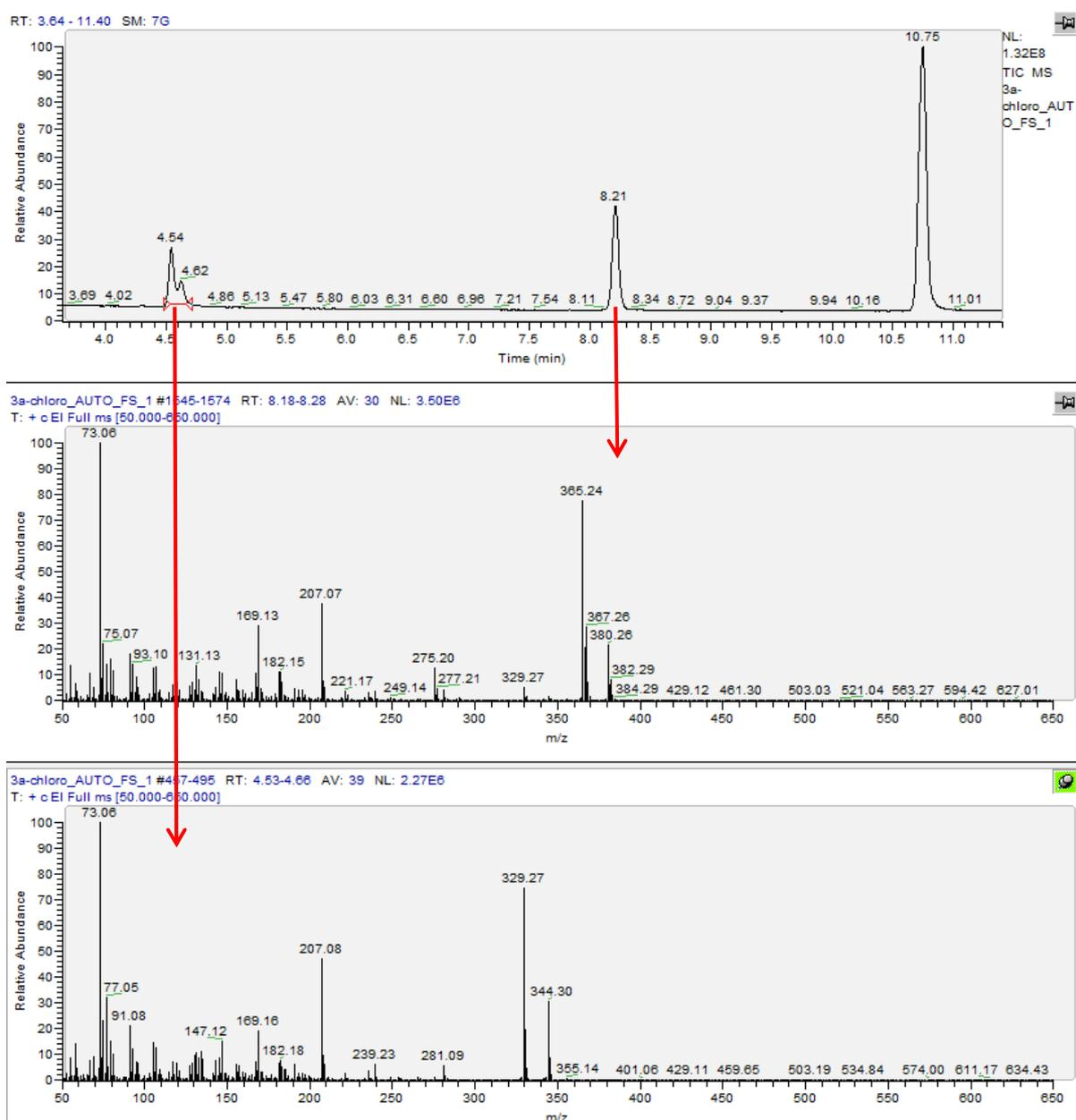
Figure 6: full scan chromatogram of internal standard *d3*-testosterone (RT 10.75), **12** (RT 8.21) and its elimination product (RT 4.54). The corresponding mass spectra for **12** and its elimination product are shown below.
