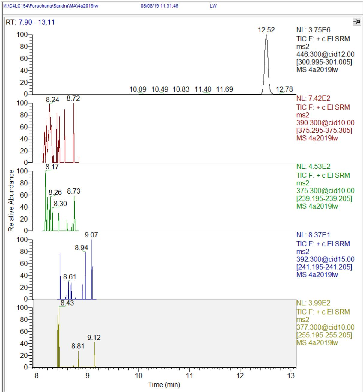
Figure 11: transition for IS methyltestosterone (RT 12.52) and selected transitions for identification for **16** (RT 8.55) and **17** (RT 8.84) of a blank water sample without **16** and **17**
