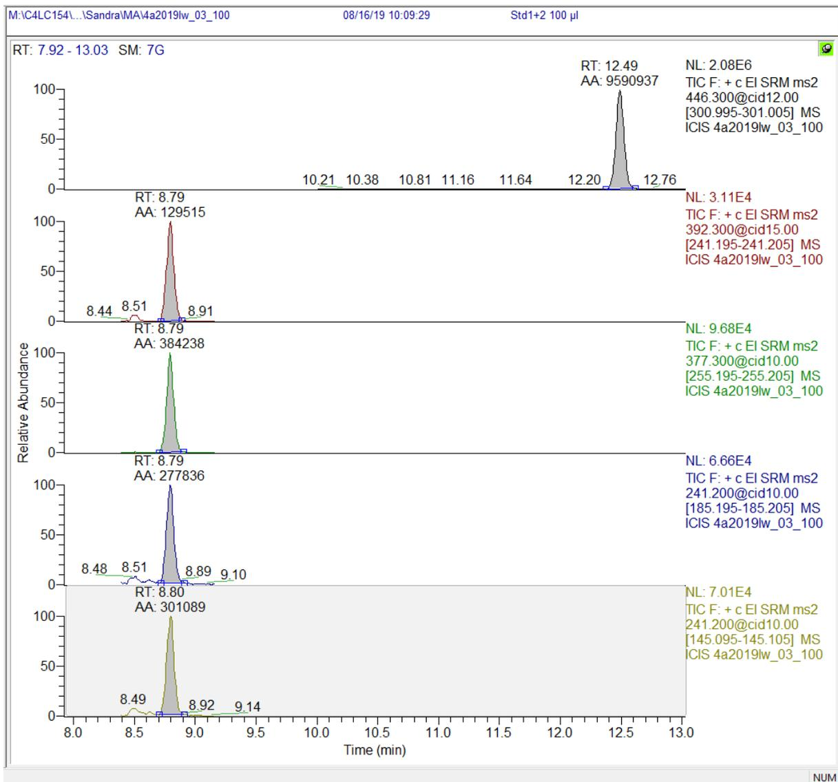
Figure 46: transition of IS methyltestosterone (RT 12.49) and four transitions for 17 (RT 8.79)
