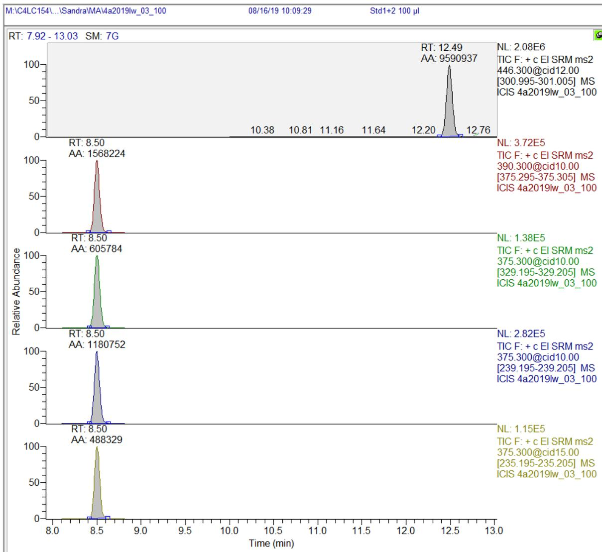
Figure 43: transition of IS methyltestosterone (RT 12.49) and four transitions for 16 (RT 8.50)
