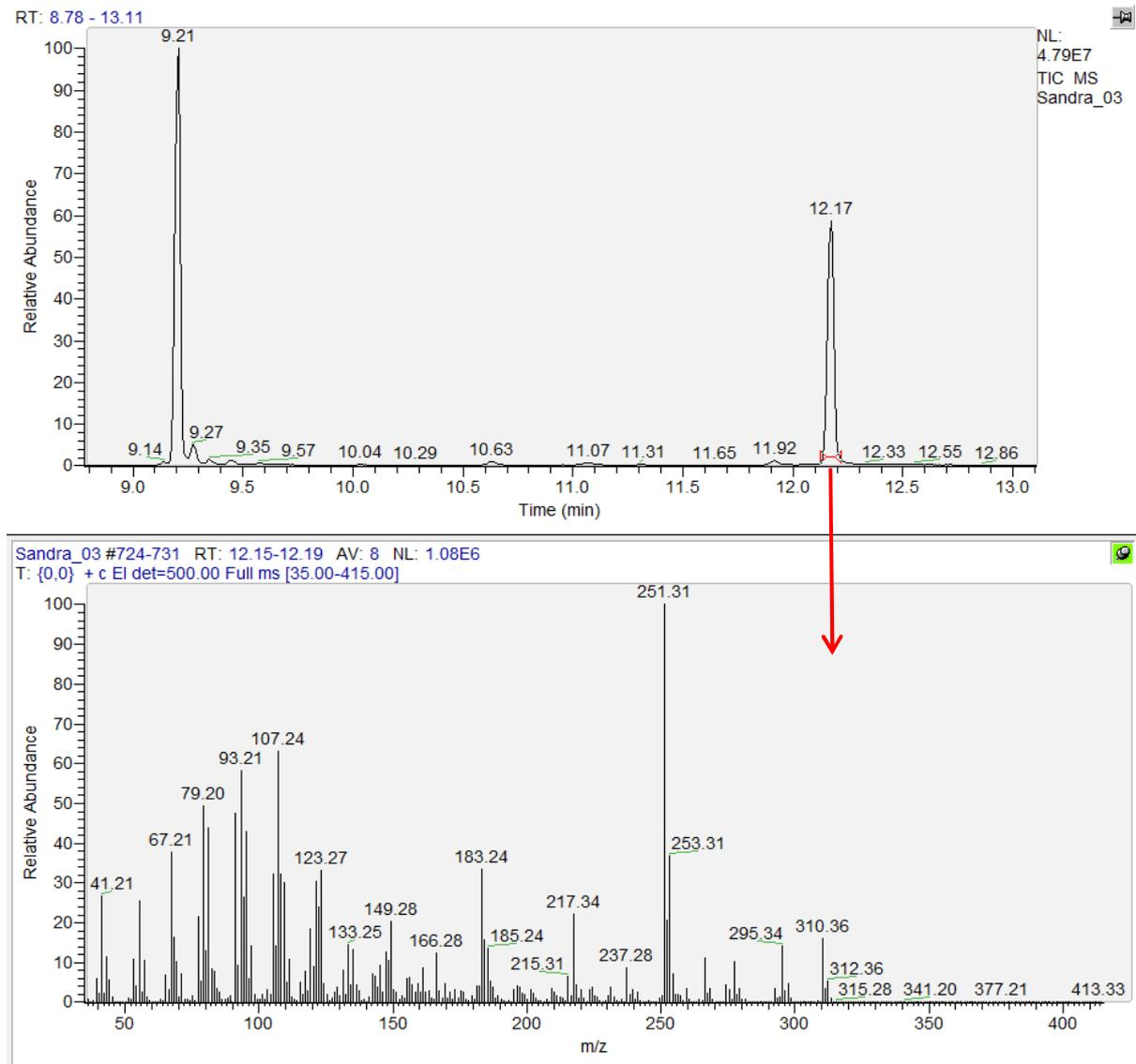
Figure 26: GC-MS chromatogram and full scan spectra of **13** without derivatization
