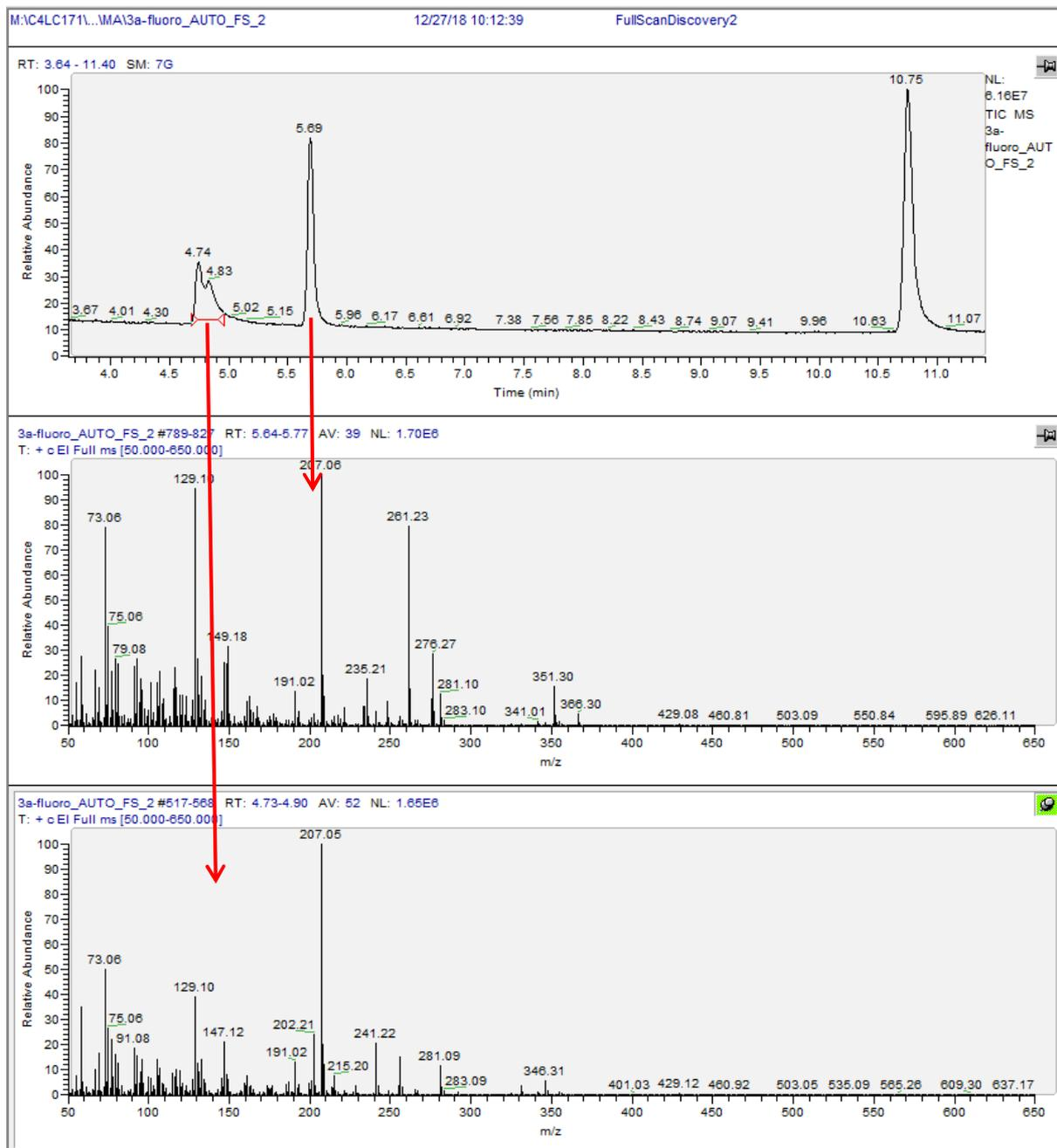
Figure 36: full scan chromatogram of internal standard  $d_3$ -testosterone (RT 10.75), **15** (RT 5.69) and its elimination product (RT 4.74). The corresponding mass spectra for **15** and its elimination product are shown below.
