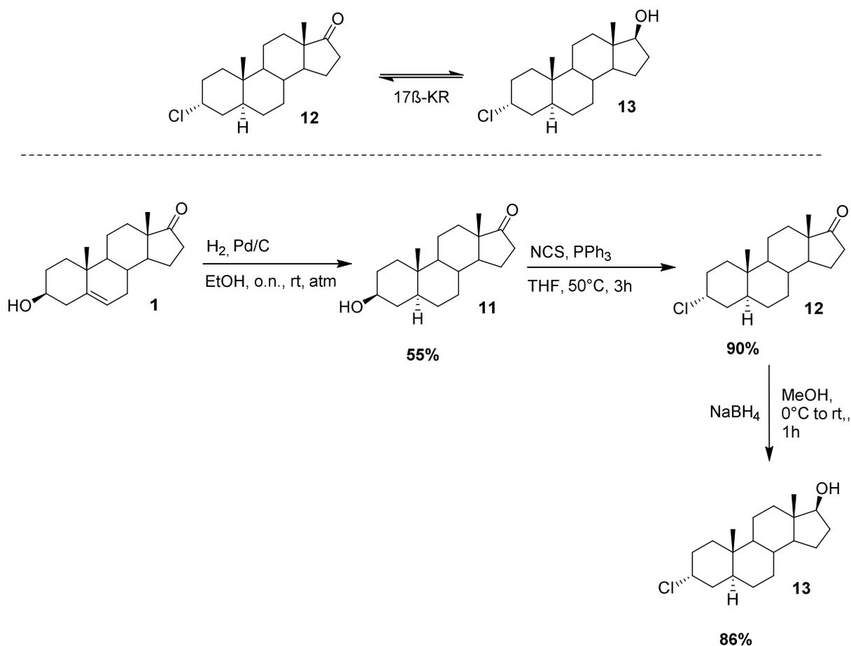
Scheme 7: synthetic route for 3 $\alpha$ -chloro-5 $\alpha$ H-androstane-17-one and 3 $\alpha$ -chloro-5 $\alpha$ H-androstane-17 $\beta$ -ol
