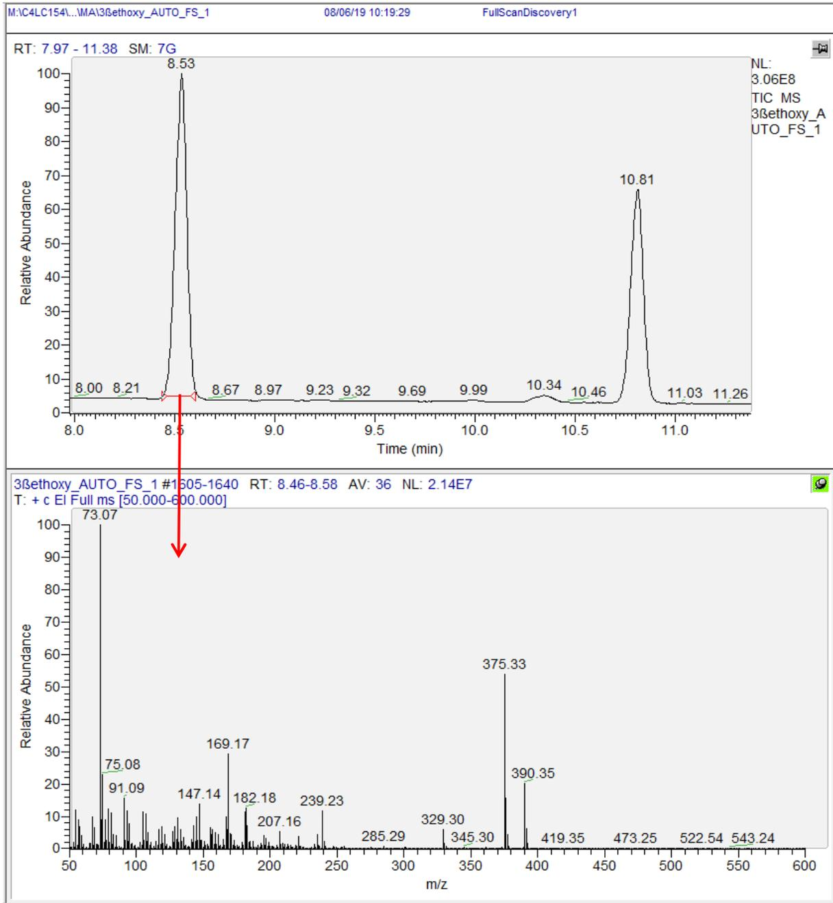
Figure 8: full scan chromatogram of IS d3-testosterone (RT 10.81) and **16** (RT 8.53). The corresponding mass spectrum for **16** is shown below.
