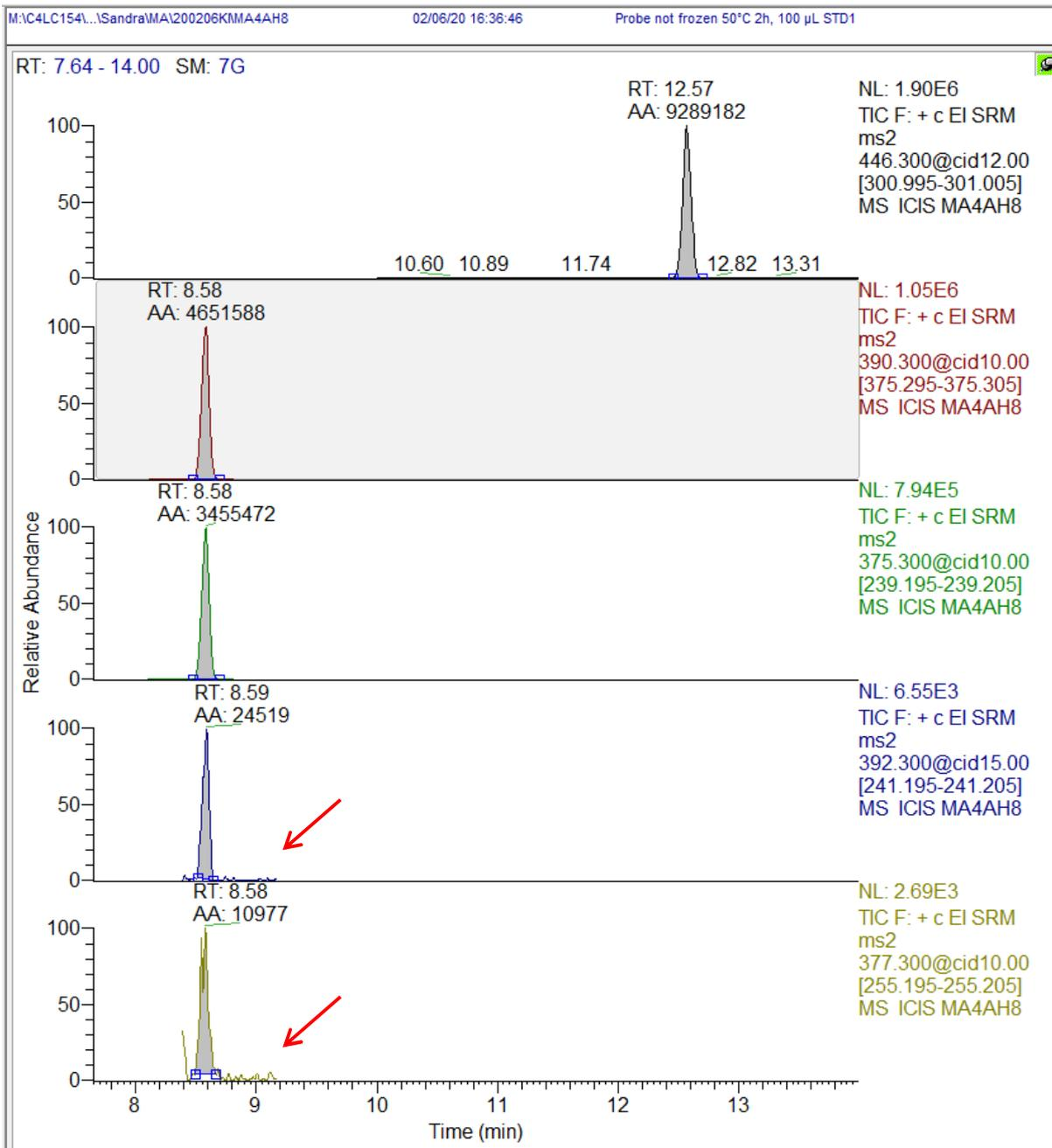
Figure 17: Preparation/analysis before freezing. Hydrolysis: Incubation 50 °C, 2 hours. Transitions for IS methyltestosterone (RT 12.57) and selected transitions for identification for **16** (RT 8.57) and **17** (RT 8.88) of a urine sample with **16** added as IS. No conversion of **16** occurred.
