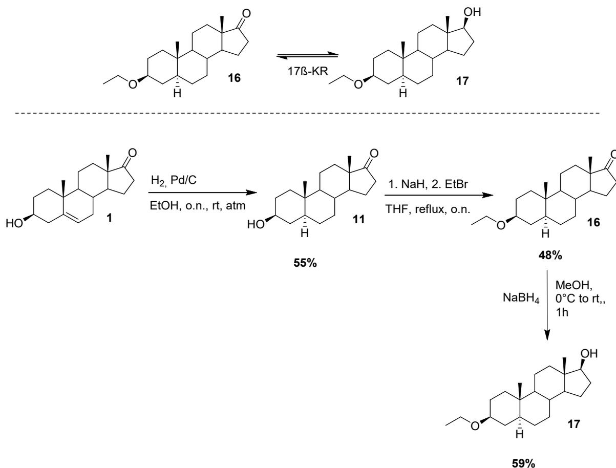
Scheme 10: synthetic route for 3 $\beta$ -ethoxy-5 $\alpha$ H-androstane-17-one and 3 $\beta$ -ethoxy-5 $\alpha$ H-androstane-17 $\beta$ -ol
