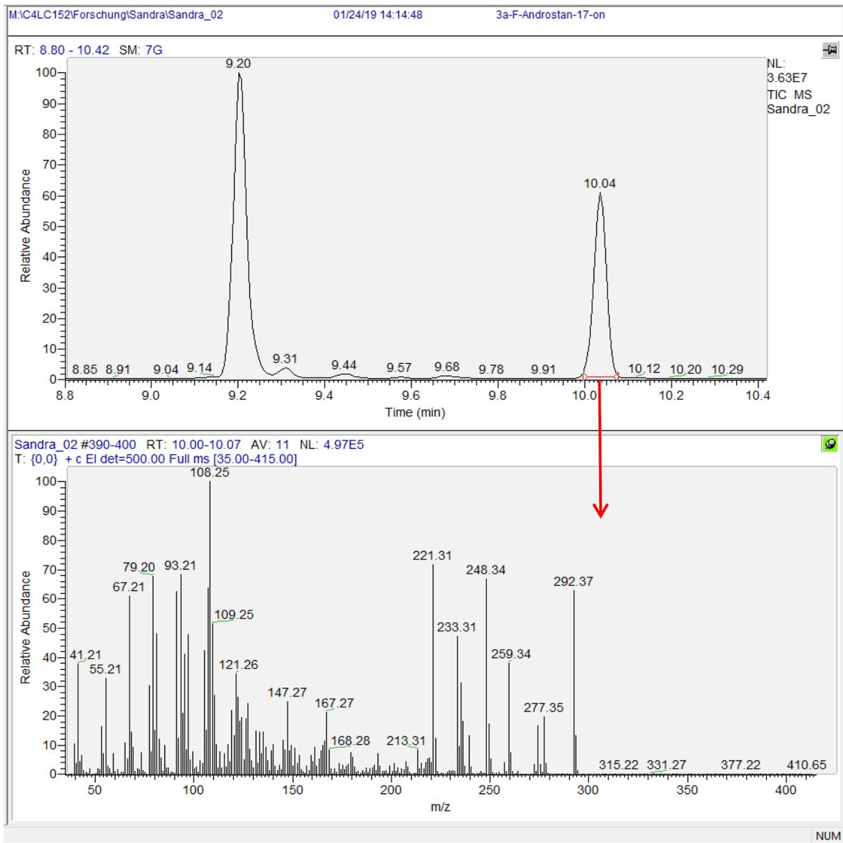
Figure 33: GC-MS chromatogram and full scan spectra of **14** without derivatization
