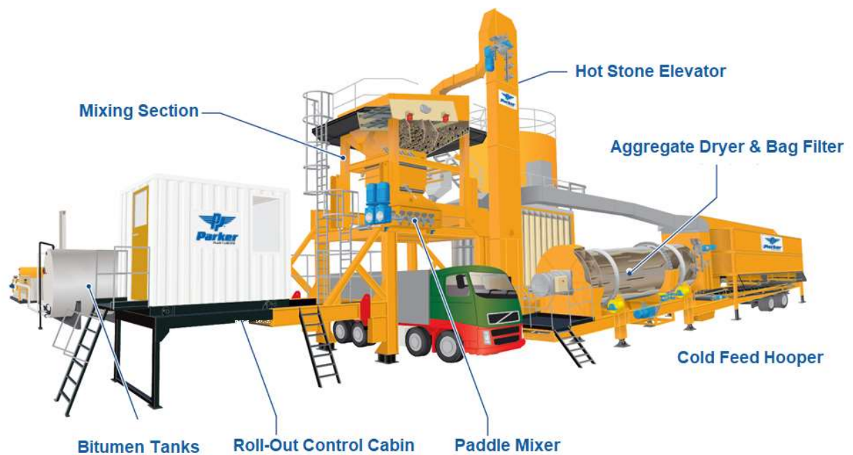
Figure 2.2 - Structure of a mobile asphalt mixing plant, RoadStar 500/1000 Mobile Asphalt Plants [1616]
