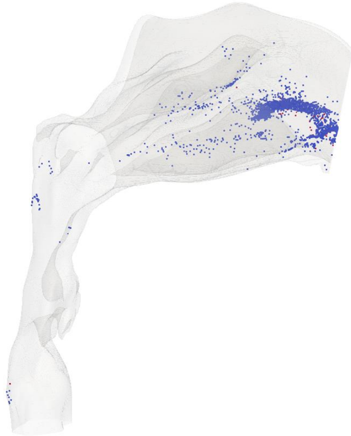
Figure 42: Particle Tracking – 50 \mu\text{m} and 15 l/min – test object A: Red – active (travelling) particles, blue – inactive (stuck) particles
