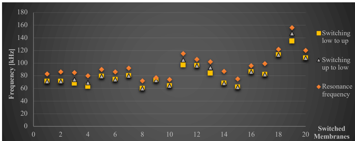
Figure 5.11: First resonance frequency and switching frequencies of every membrane, which was able to achieve required switching displacements. Membranes 1 – 10: 800 \mu\text{m} diameter; 11 – 17: 700 \mu\text{m} diameter; 18 – 20: 600 \mu\text{m} diameter.
