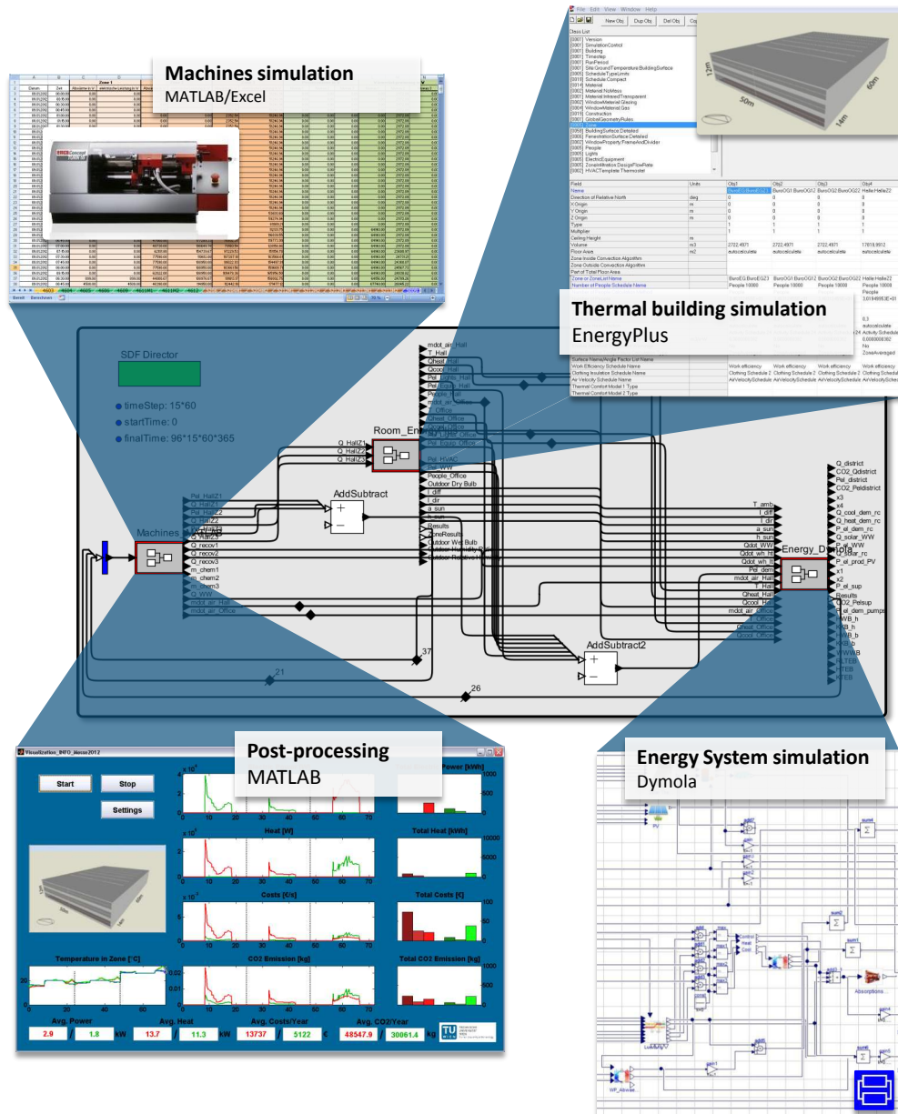
Figure 3.6: Overall co-simulation implementation for the case study, including MATLAB, Dymola and EnergyPlus simulations, coupled via BCVTB middleware [130].
