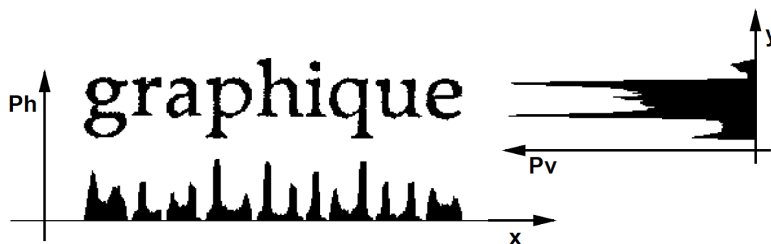
Figure 2.7: Horizontal (Ph) and vertical (Pv) projection profile of the word graphique , courtesy by [ZI93].
