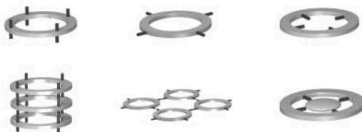
Figure 5: Different orientations of the side groups (functional groups) that are attached to the macrocycles lead to distinctive motifs after self-assembly [13]
