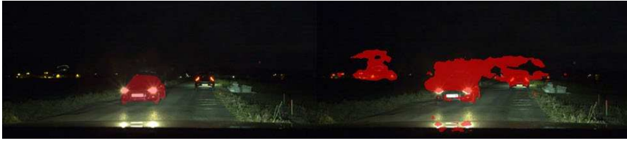
Figure 2.4: (left) correct mask of oncoming traffic, (right) falsely propagated mask of oncoming traffic by OSVOS network.
