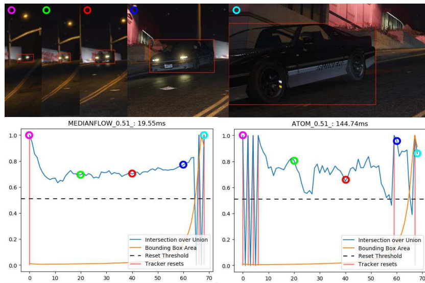
Figure 5.4: Scene (top) with oncoming traffic. ATOM (bottom right) has problems when car is still small and only headlights are visible. MedianFlow (bottom left) delivers more stable tracking results in this situation.
