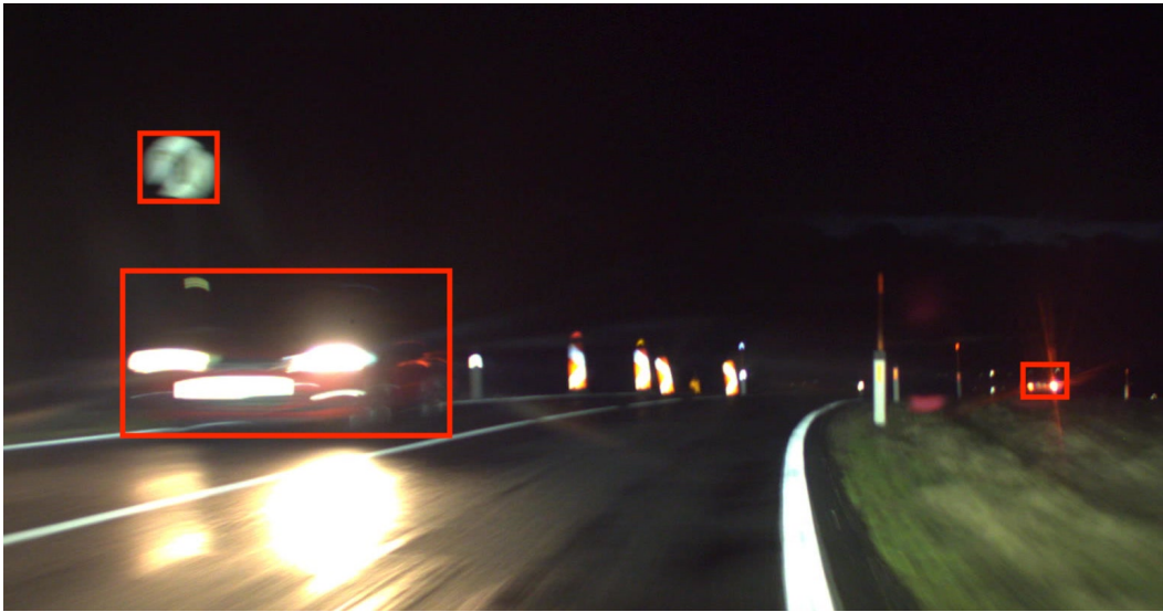
Figure 3.19: Examples of motion blur (left car, traffic sign) and lens flare (right car).
