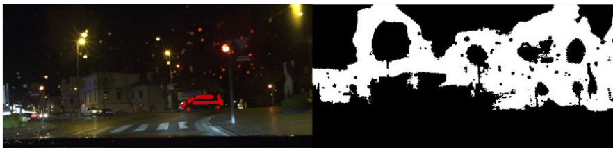
Figure 2.3: Left: a test image from our nighttime road scenes. Right: the filtered foreground region, showing that CVF in this case does not deliver meaningful results.
