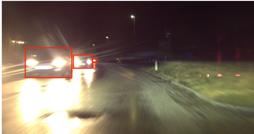
Figure 3.17: Over-exposure (white reflection on road) and lens flares (star-shaped streaks around headlights, red dots on grass patch).
