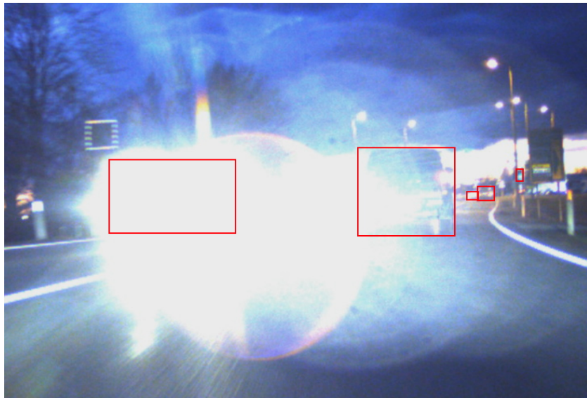
Figure 3.18: Over-exposure and lens flare of oncoming headlight affecting almost the entire field of view.
