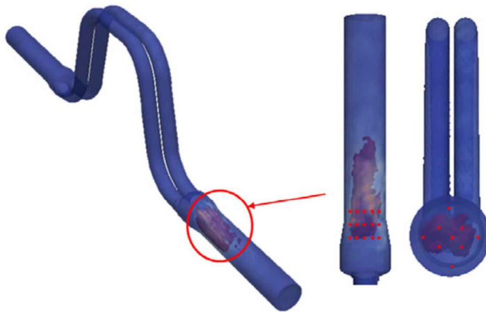
Figure 6.4: The monitoring points (in red) used to build the turbulence energy spectrum from the velocity vectors in the high device.
