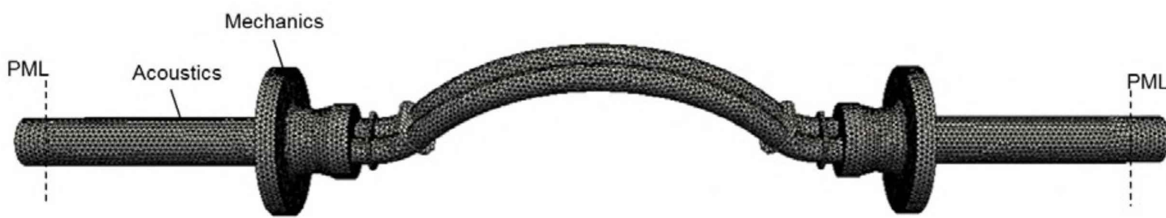
Figure 3.5: An example of the vibroacoustic mesh of the compact geometry with acoustic, mechanical and boundary regions.
