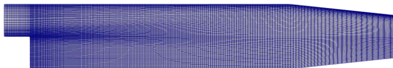
Figure 3.16: Pitz-Daily computational mesh
