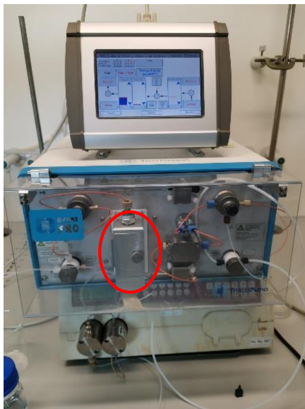
Figure 15: The H-cube ® apparatus with an external pump and reaction chamber containing the Pd hydroxide catalyst circled in red.
