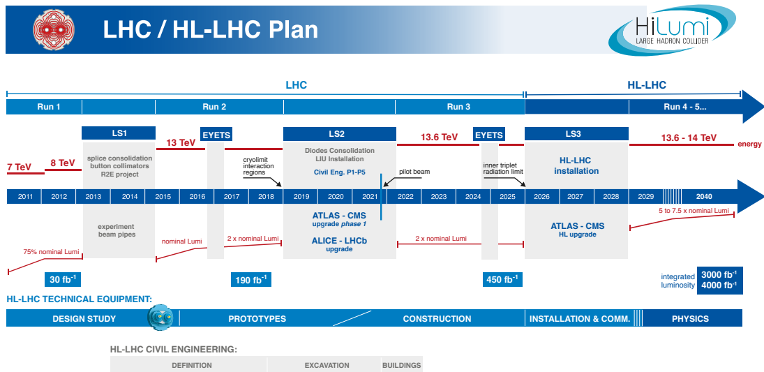
Figure 2: LHC schedule including the plan for the HL-LHC upgrade. Taken from [8].
