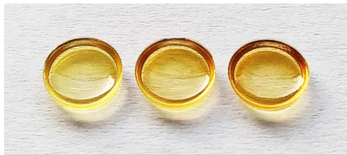
Figure 48: Poly(BisOx) photopolymerized with 1 mol% S-B at 140 °C
