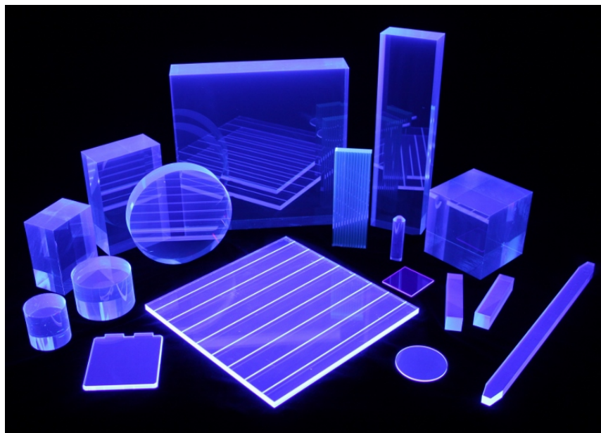
Figure 2.9: Commercially available plastic scintillators [23].
