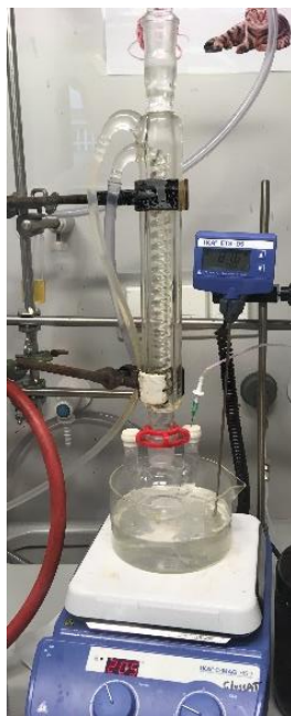
Figure 3-18 Cyclohexane oxidation reaction set-up
